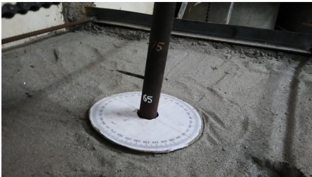
Fig 4.3: pile inserted inside sand to 60cm of depth
