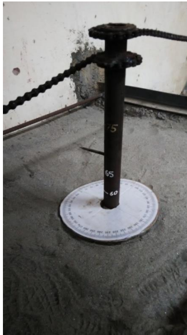
Fig4.2: pile inserted inside sand to 55cm of depth
