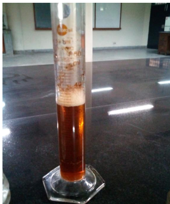
Figure 3.6: Metal ion extraction from leachate by addition of nitric acid
