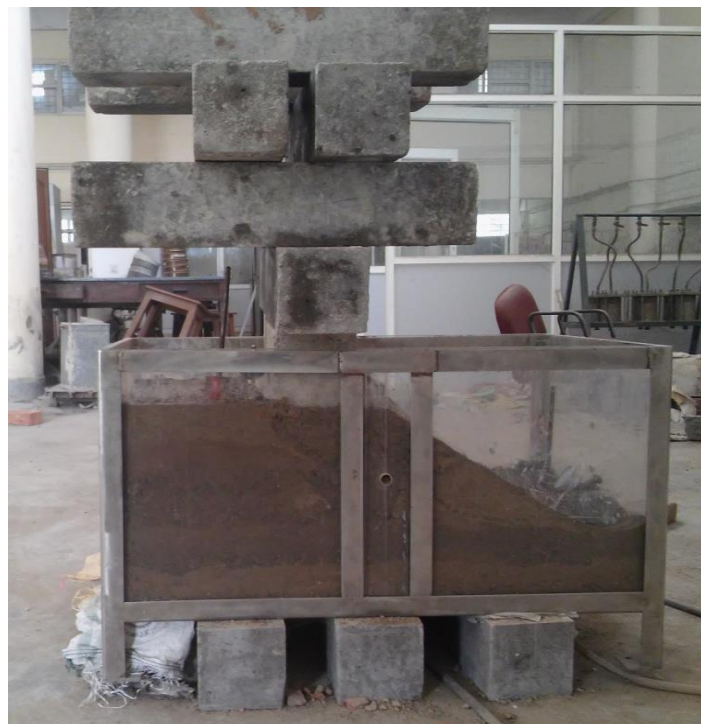
Fig.5 Model with slope failure
