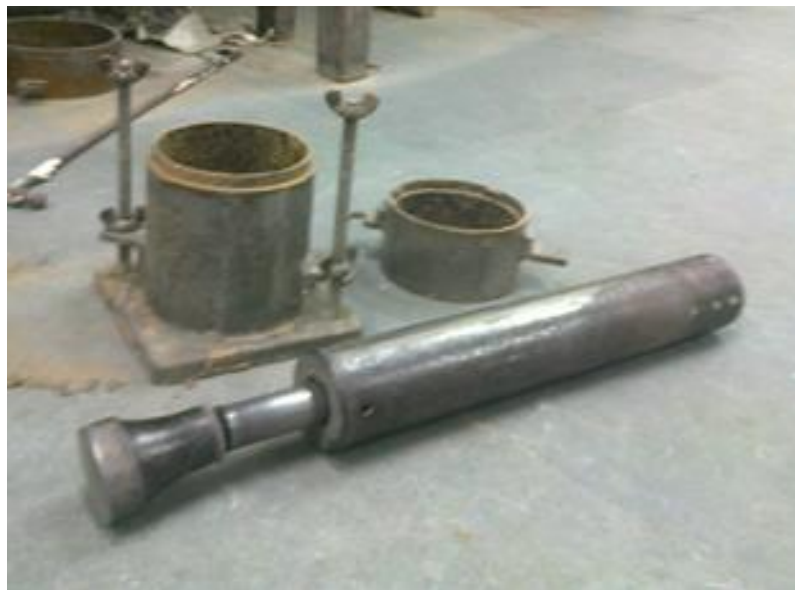
Fig.11 standard proctor apparatus
