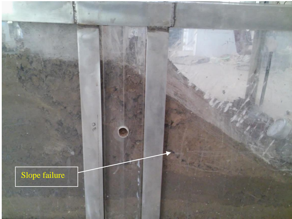
Fig.6 Model with failure surface
