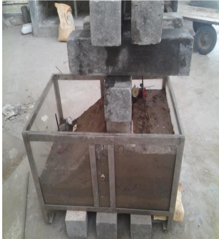
Fig.4 Model with gravity loading(Max. 1400 Kg)
