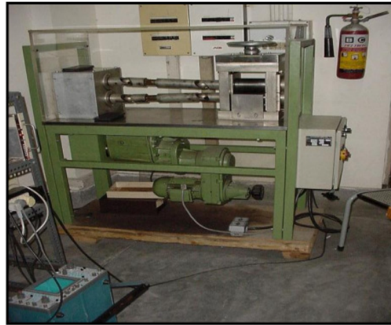
Figure 2.3: The rolling machine used for the preparation of thin samples and catcher foils at the target laboratory of IUAC.
