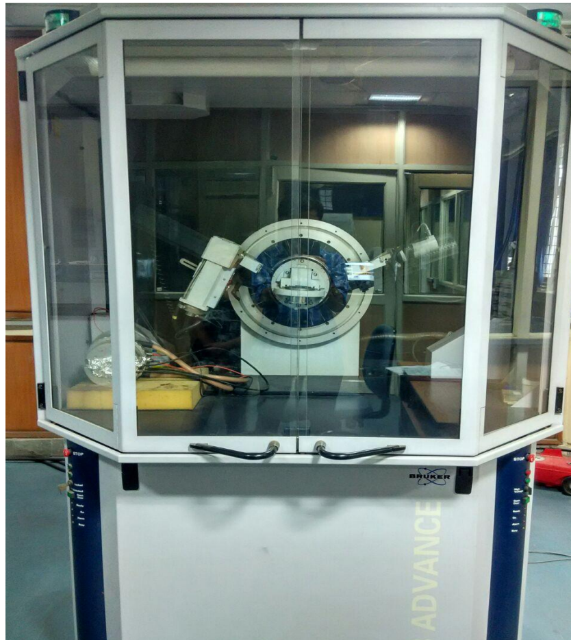
Fig 5.2 Picture of XRD set up @DTU
