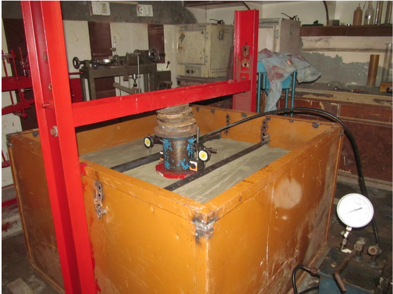
Figure 1: Set up of plate load test.
