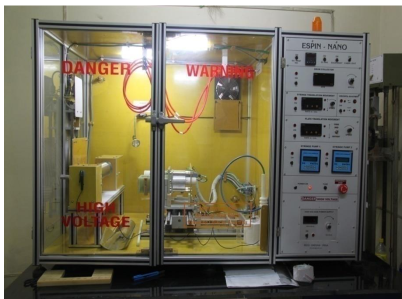
Figure 2.1: Setup of an electrospinning unit (ESPIN-NANO (PHYSICS EQUIPMENT CO.))
