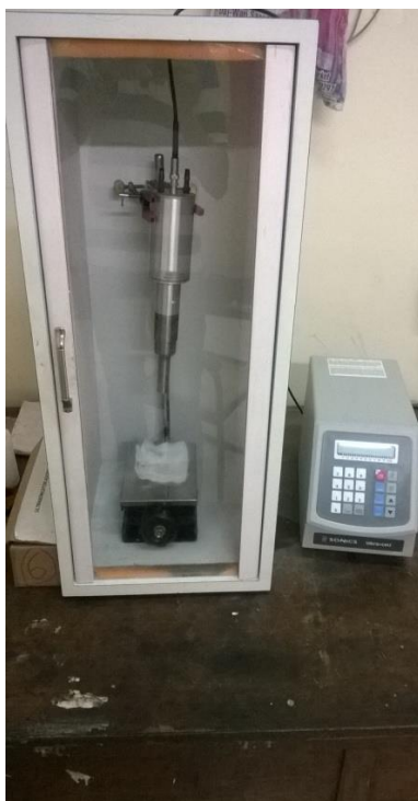
Figure2.3: Ultrasonicator used for dispersion of MOF-5 in polystyrene solution
