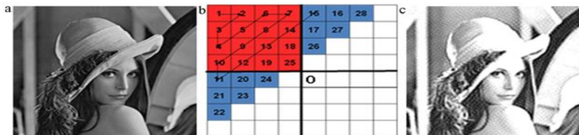
Fig. [a] the Lena image (b) Zigzag order scanning (c) the reconstruction image of Lena by using 1/4 DCT coefficients.
