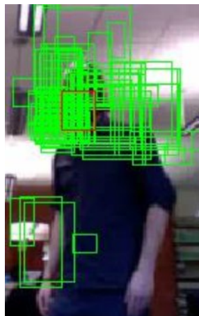
Fig 3.11 Example of a multimodal particle set tracking a face, but also caught onto an arm
