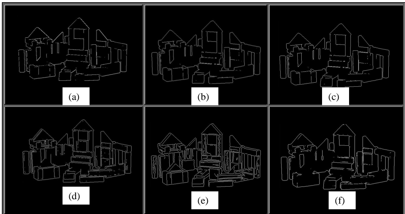
Figure 23. The results of different edge detectors on Sunflower image (a) Roberts (b) Sobel (c) Prewitt (d) Laplacian of Gaussian (e) Canny (f) Proposed
