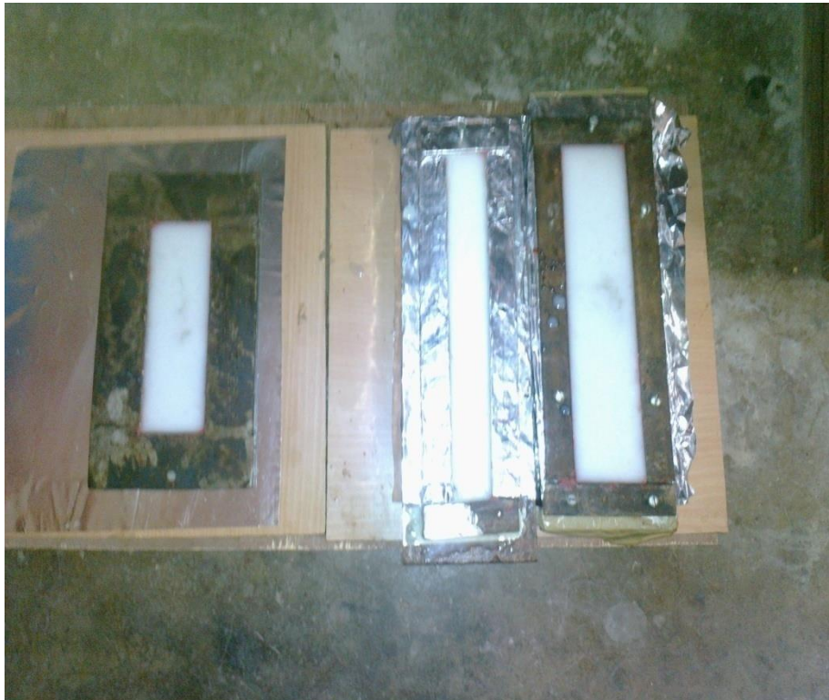
Fig.3-The mold has a 300*300*5mm dimension.
