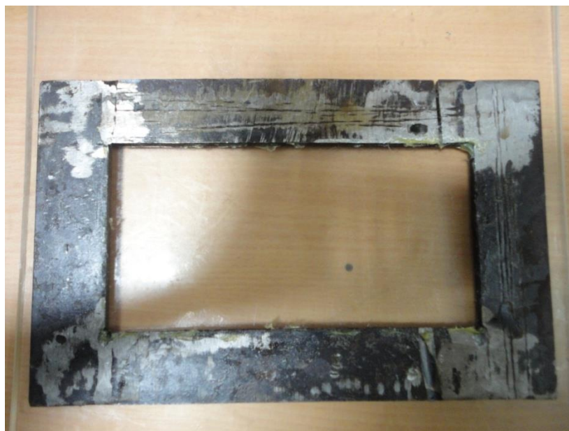
Fig.2 Mold Used for preparing flate 5 mm thick cured Epoxy/PVAC sheet
