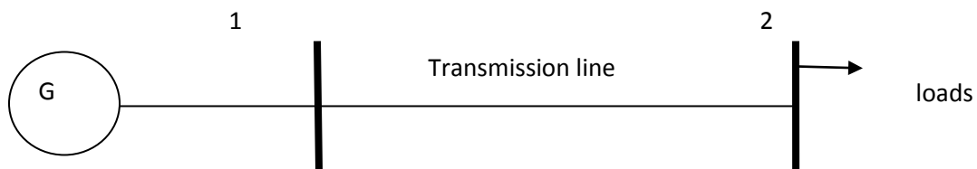
Fig 4.1 Simple model of power system
