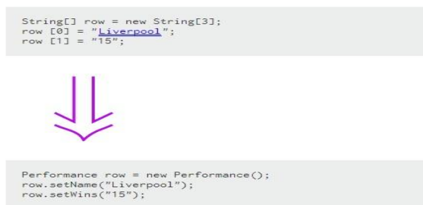
Figure 8: Replace Array with Object
