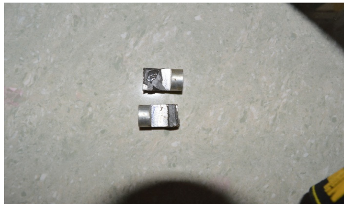
Fig 3.7- Failure of adhesive in lap joint specimen during dynamic test.
