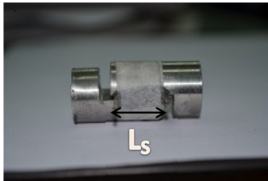
Fig-3.2-Aluminium-6063 T6 specimen for dynamic compression test.
