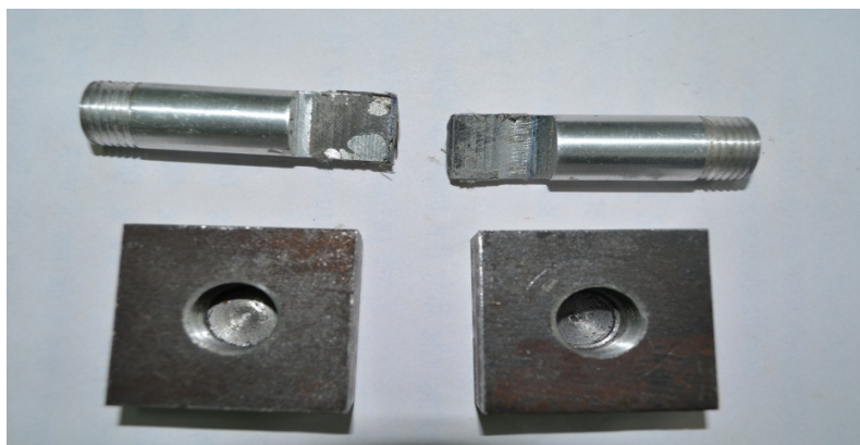
Fig 3.4-Adhesive failure of the joint in static compression test and specimen holder.
