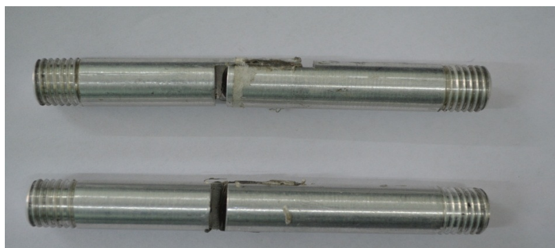
Fig 3.1-Aluminium-6063 T6 specimen for static test.
