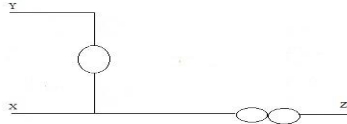
Fig 2.7 A Simplified representation of CCII-
