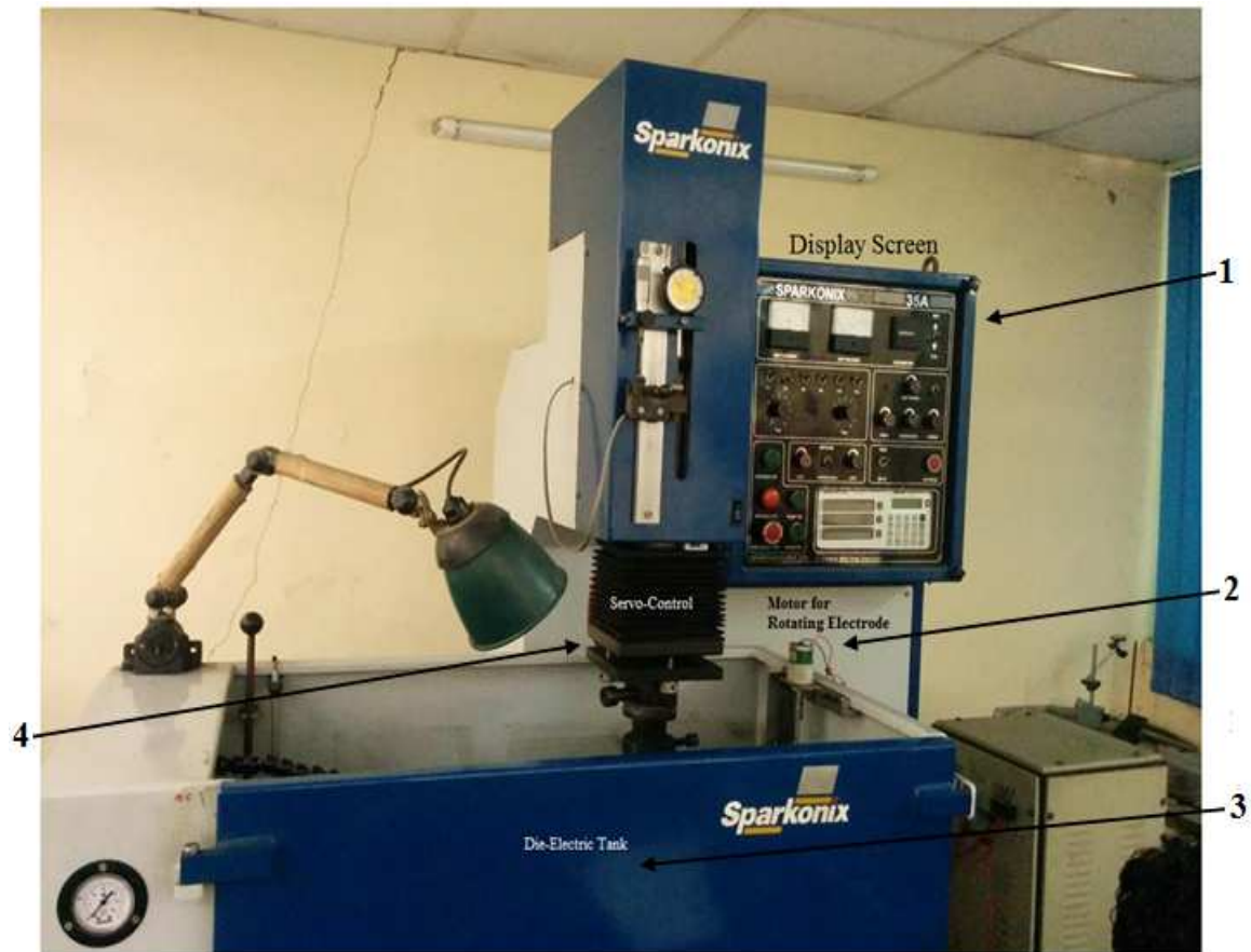
Figure 4.2: HEDME Machine Tool (1: Display Motor. 2: Motor for Rotating Mechanism, 3: Die-Electric tank, 4: Servo-Control)
