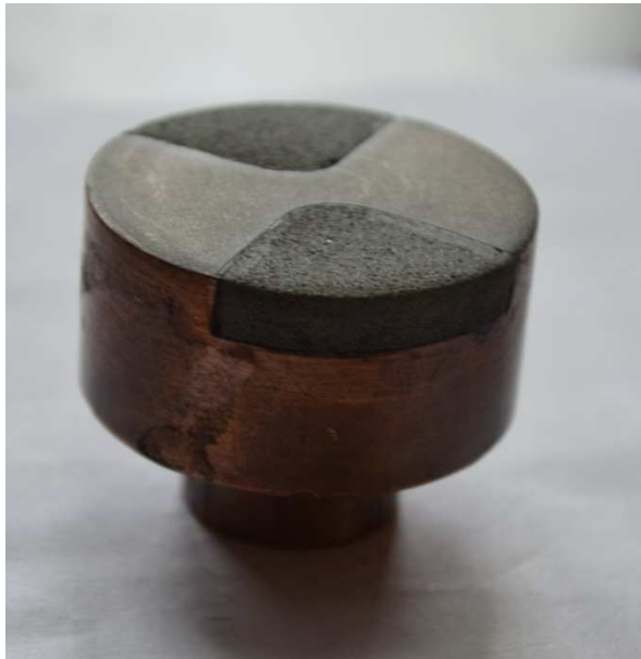
Figure 5.6: Specimen of 3 rd design of Developed Hybrid EDM Electrode of Copper
