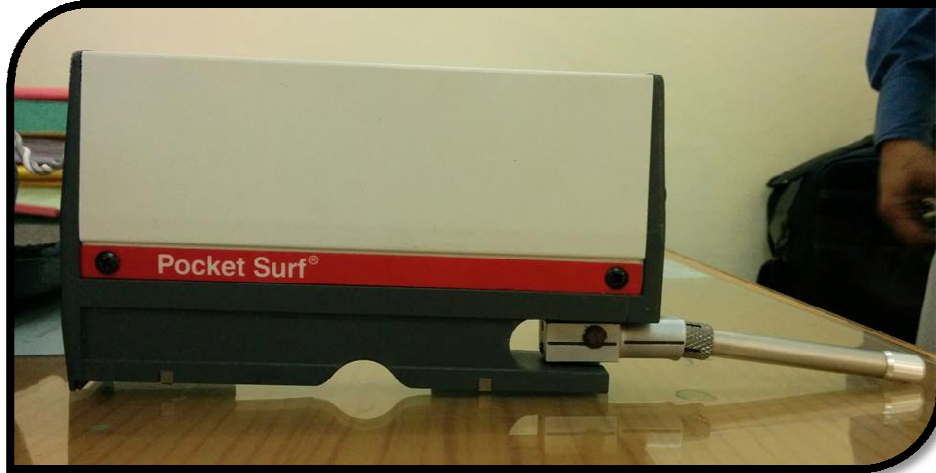
Figure 5.9: Surface Roughness Tester [Mahr Federal (Model: Pocket Surf III)]
