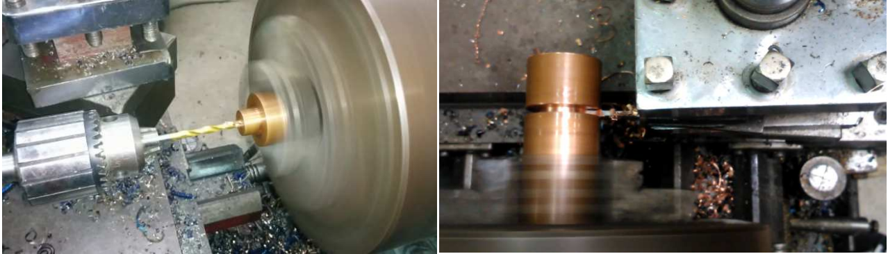
Figure 5.2: Turning Processes on Electrode
