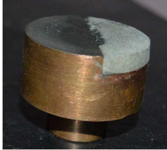
Figure 5.5: Specimen of 2 nd design of Developed Hybrid EDM Electrode of Copper
