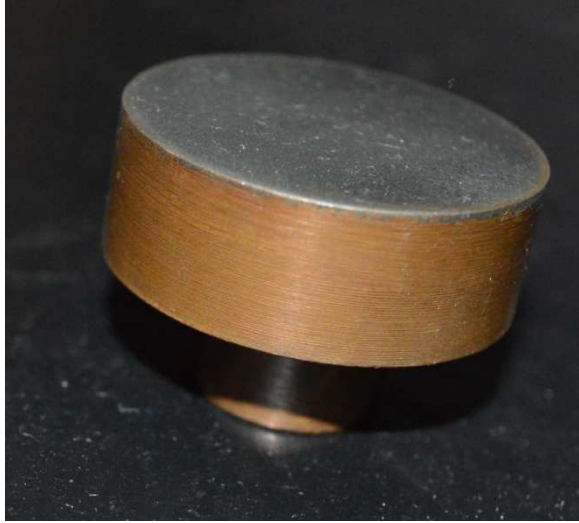
Figure 5.4: Specimen of 1 st design of Developed Hybrid EDM Electrode of Copper
