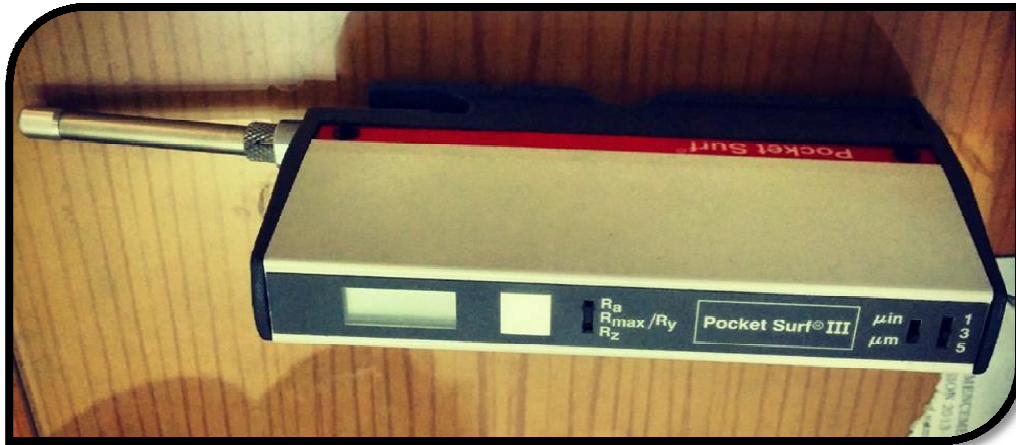
Figure 5.10: Surface Roughness Tester showing its various measuring range [Mahr Federal (Model: Pocket Surf III)]
