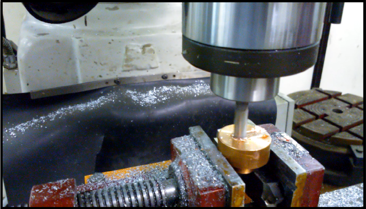
Figure 5.3: Milling Processes on Electrode
