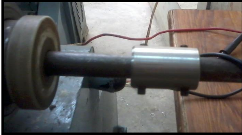
Figure 3.23 Coupling joining the iron rod and the mercury box
