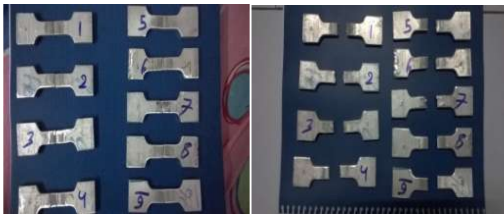
Figure 3.23 specimens for tensile test
