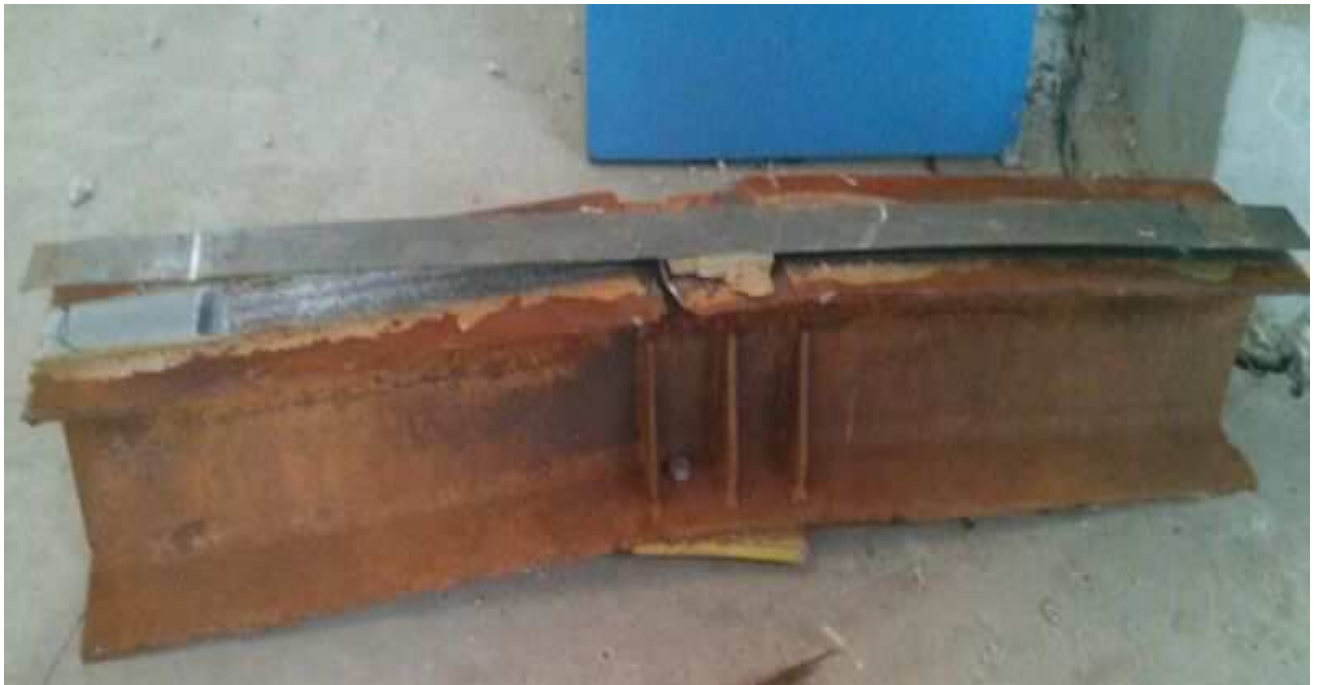
Figure 25 a): Beam 2 after test showing mode of failure complete steel and adhesive interface debonding.
