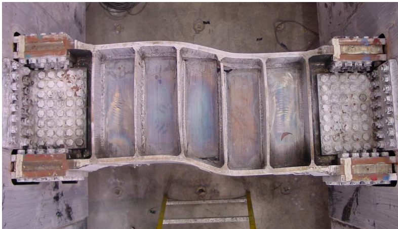
Figure 3: Shear Links for Seismic Retrofit [3]
