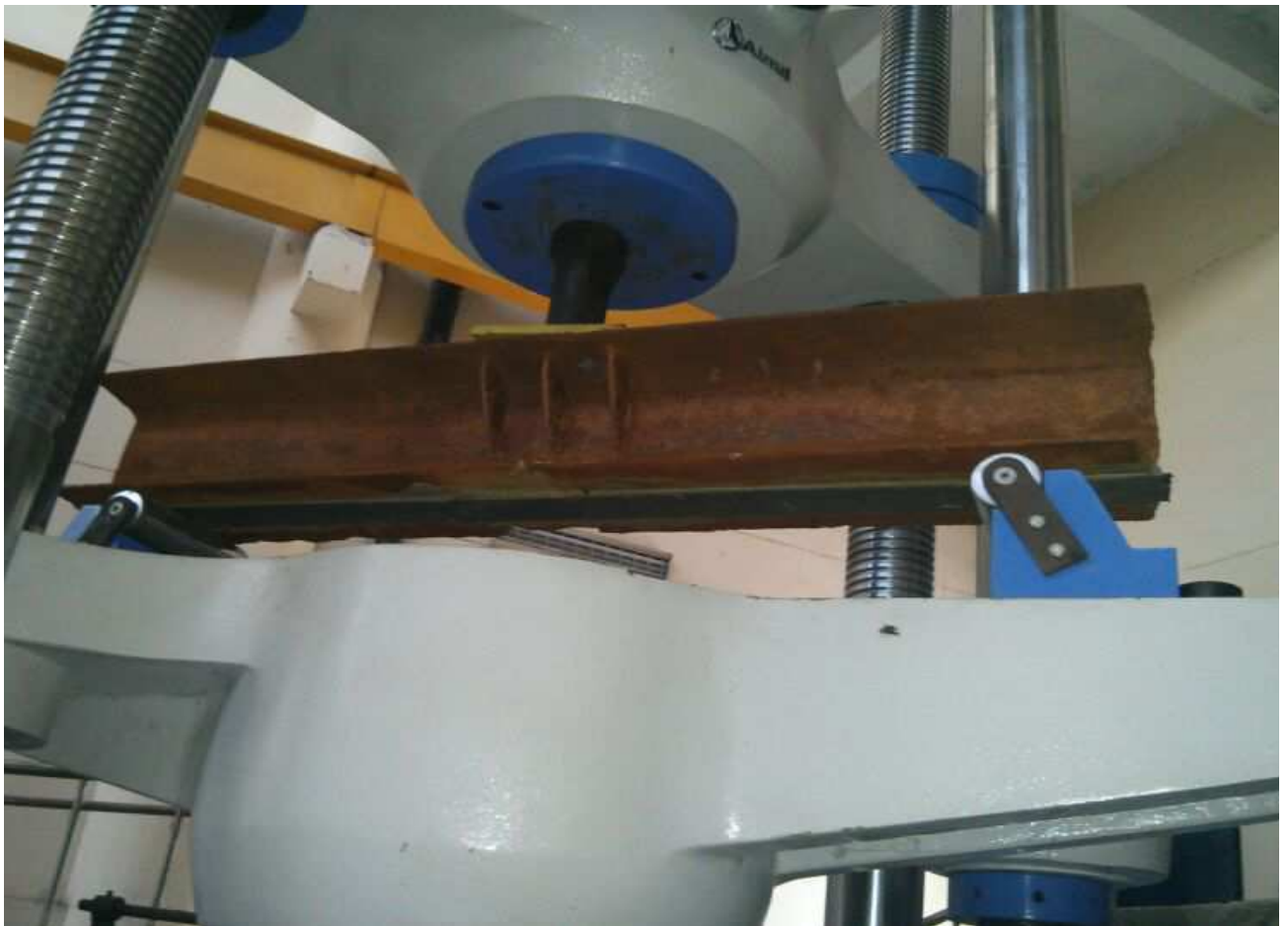
Figure 21: Beam 2 before test in position for testing on Universal Testing Machine.
