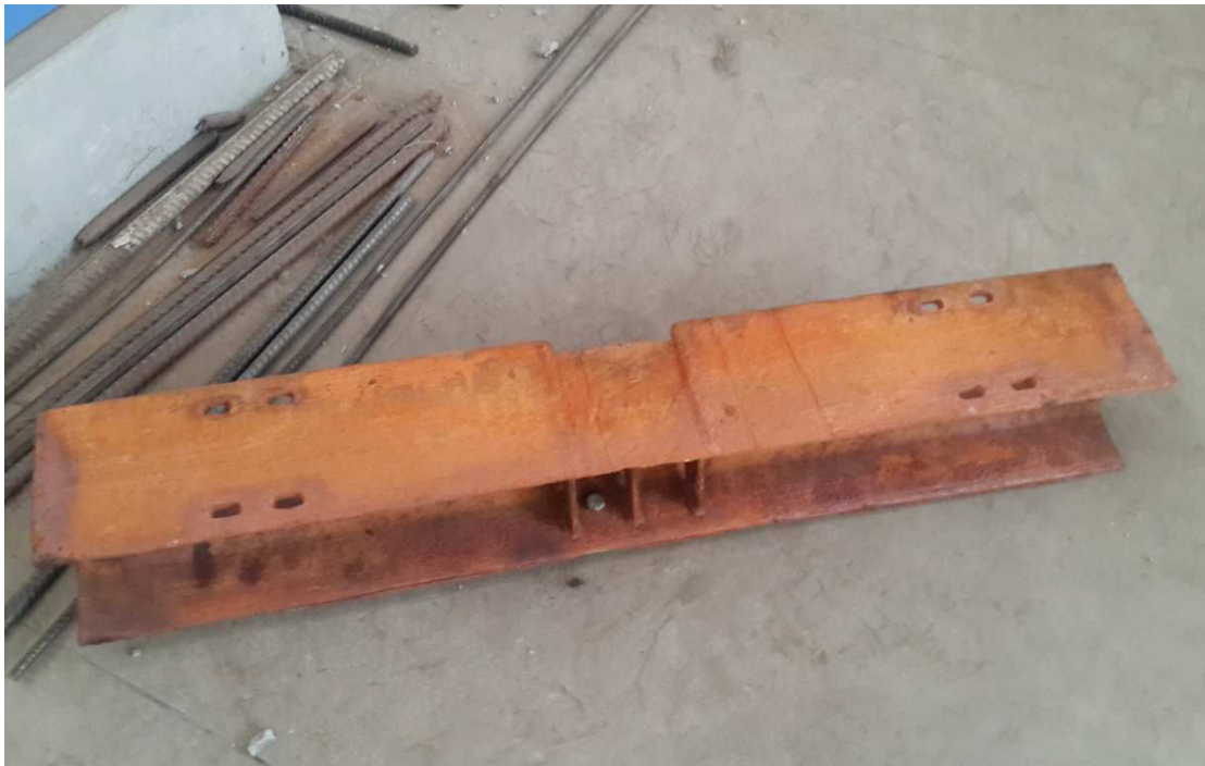
Figure 17: Typical beam after corrosion
