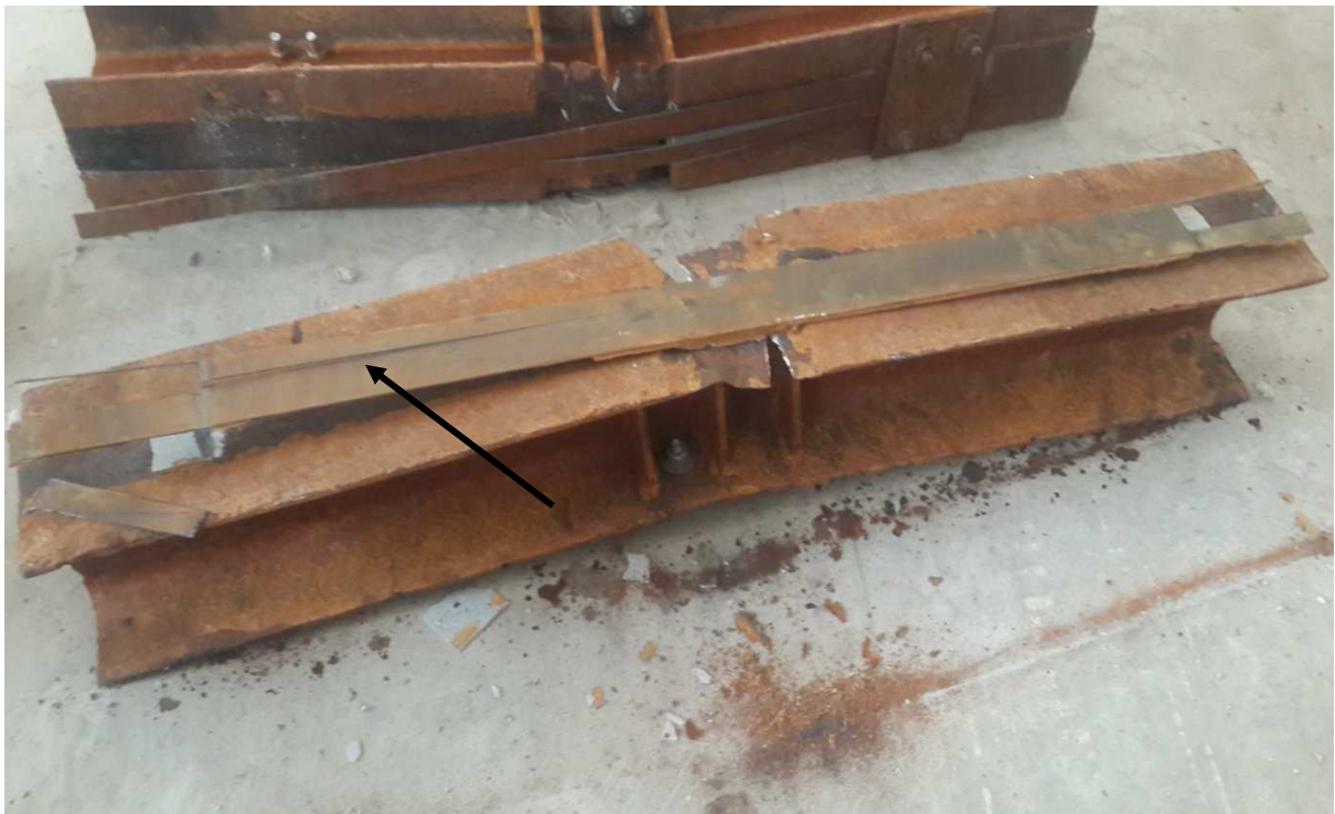
Figure 25 c): Beam 4 after test showing mode of failure i.e. CFRP tensile rupture
