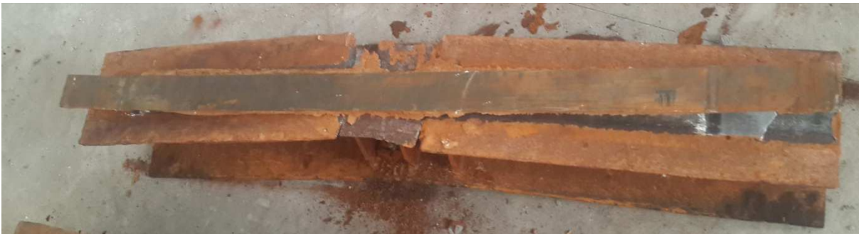
Figure 25 d): Beam 5 after test showing mode of failure complete steel and adhesive interface debonding failure.
