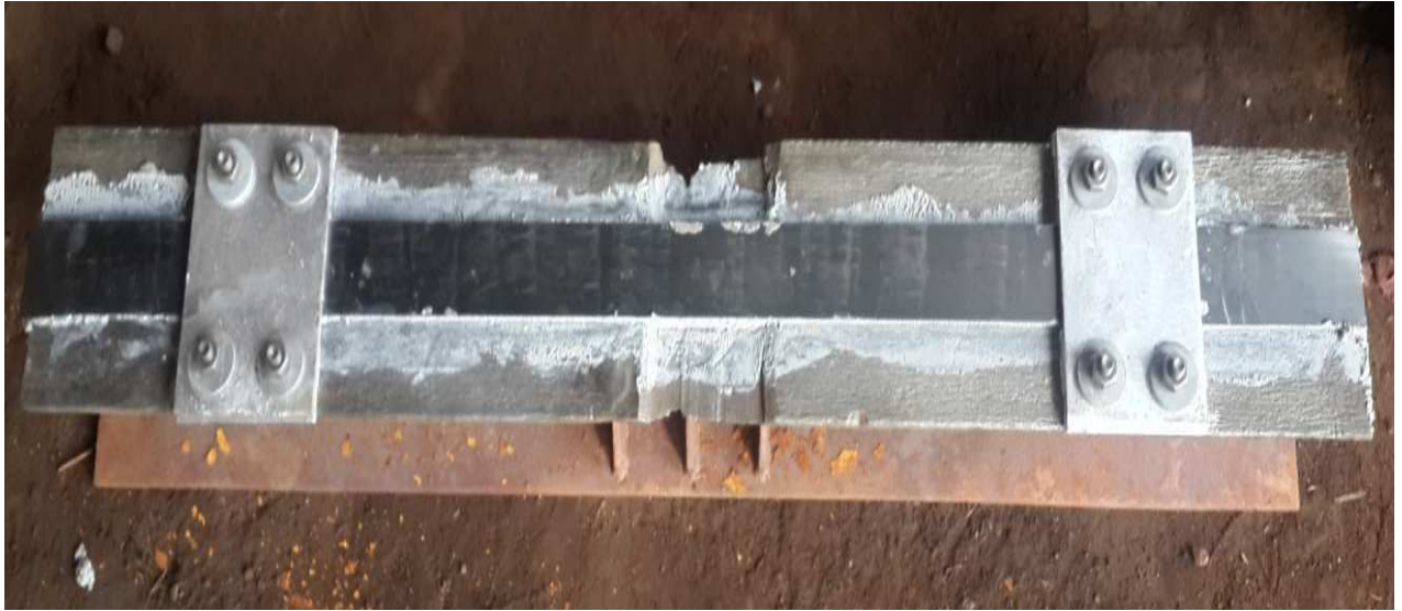
Figure 20: Typical Beam strengthened with CFRP and end-anchor plates.
