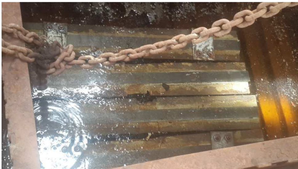
Figure 23: Beams immersed in saline water tank
