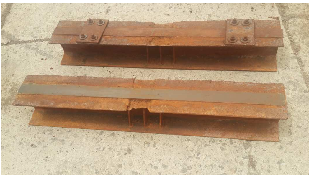
Figure 24 b) : Beam 5 and Beam 8 after exposure in saline water tank for 30 days and giving daily one wetting-drying cycle.
