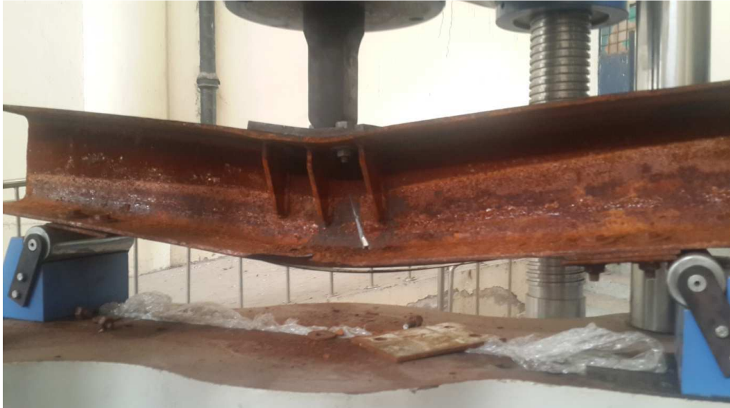
Figure 25 f): Beam 7 after test showing mode of failure CFRP tensile rupture.
