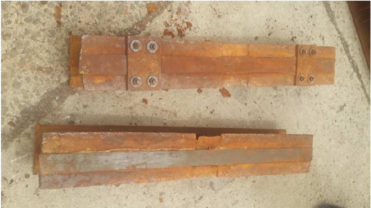
Figure 24 a) : Beam 4 and Beam 7 after exposure in saline water tank for 30 days and giving daily one wetting-drying cycle.
