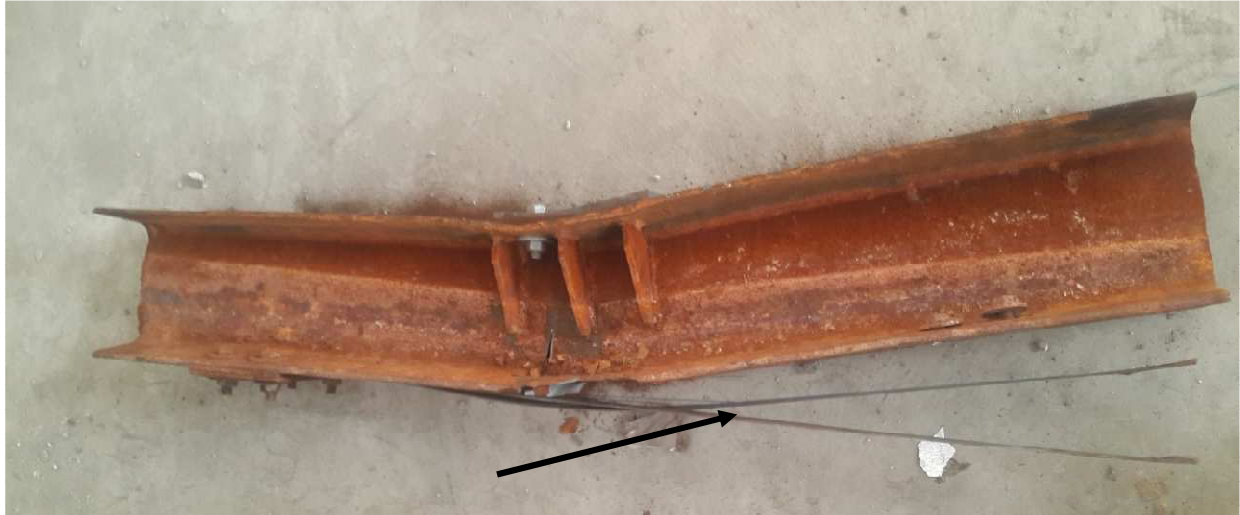
Figure 25 h): Beam 9 after test showing mode of failure CFRP tensile rupture along with End Anchorage Failure
