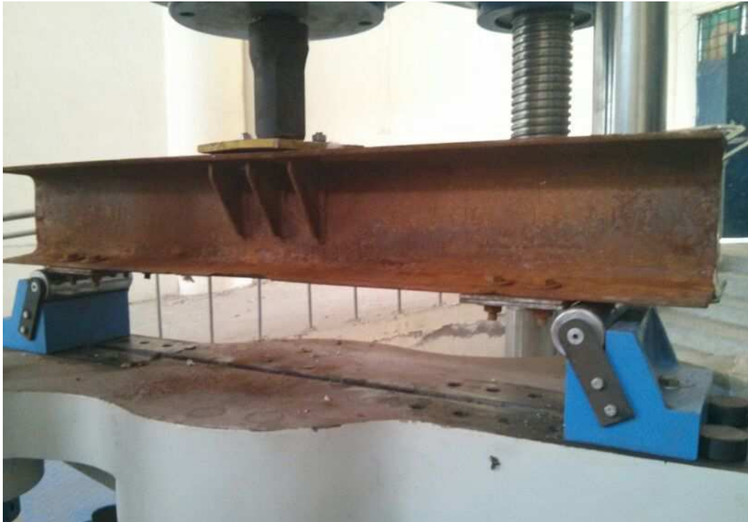
Figure 22: Beam 3 before test in position for testing on Universal Testing Machine (UTM)
