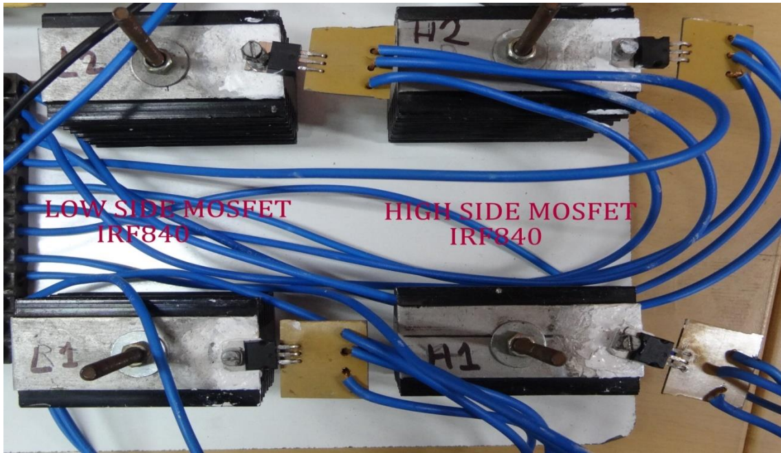
Figure 4-16 Developed hardware for Power Circuit
