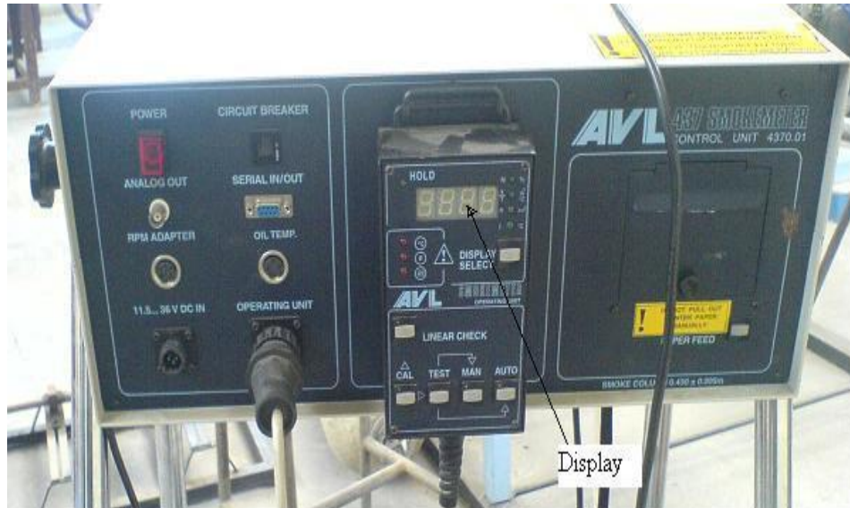
Figure 5.3 An AVL Smoke meter
