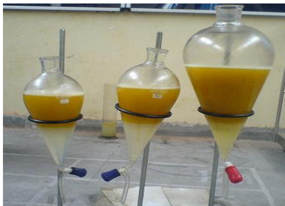
Figure 3.2: Washing process of biodiesel
