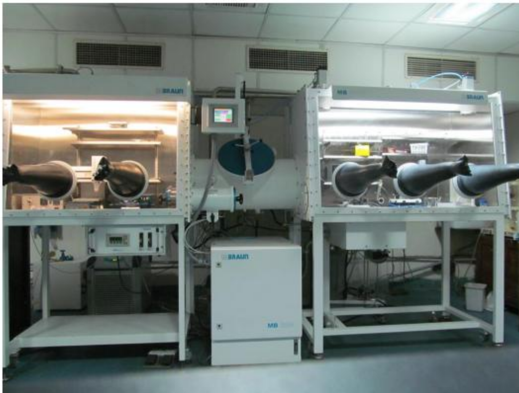
Figure 3.5 Automated Glove Box System with Metallization compartment and Spin coating compartment (NPL, New Delhi)
