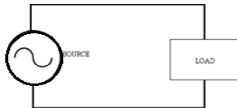
Fig. 5.2 AC source and an electrical load
