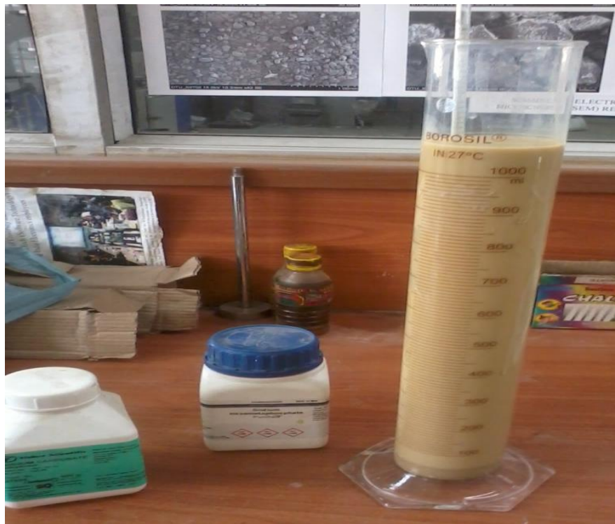
Figure 4.1: Grain size analysis through hydrometer
