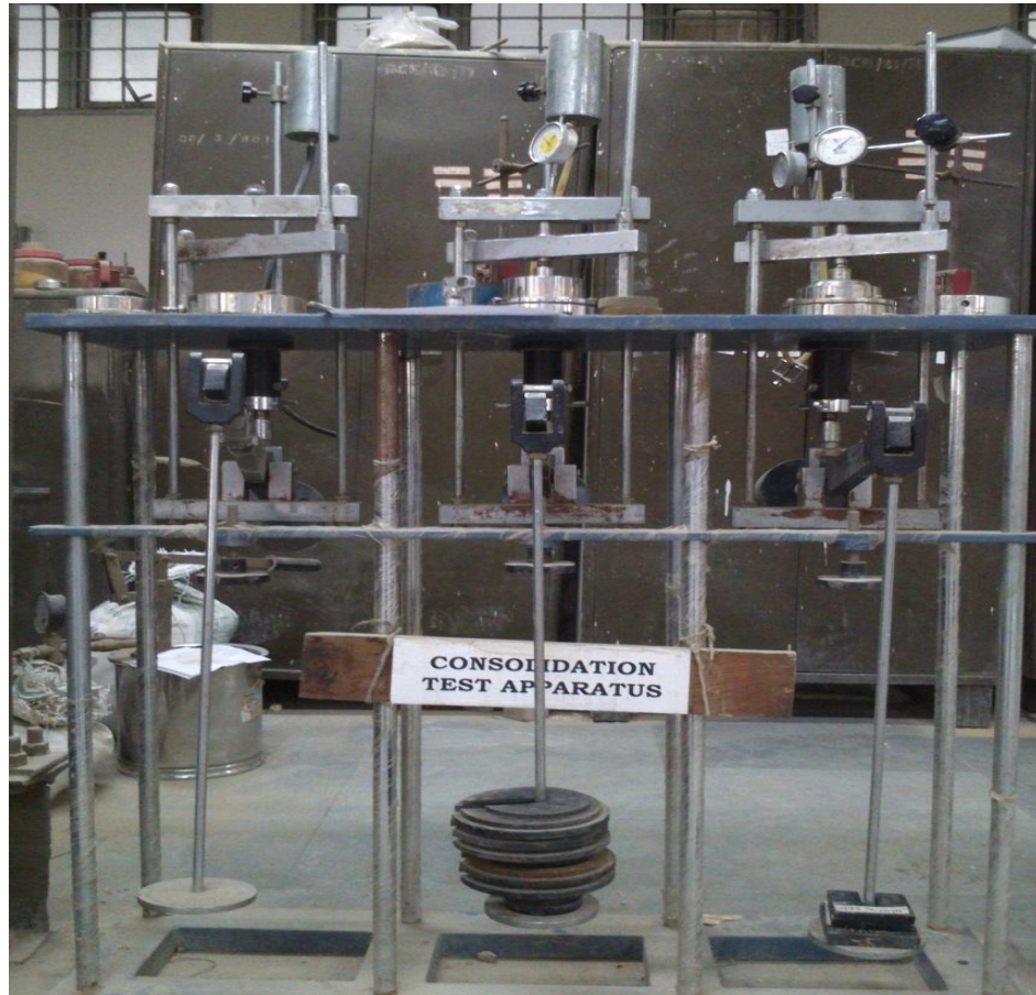
Figure 4.4:- Consolidometer Test Apparatus at loading
