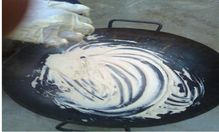
Figure 5.2: Al 2 O 3 abrasive particle mixed with media
