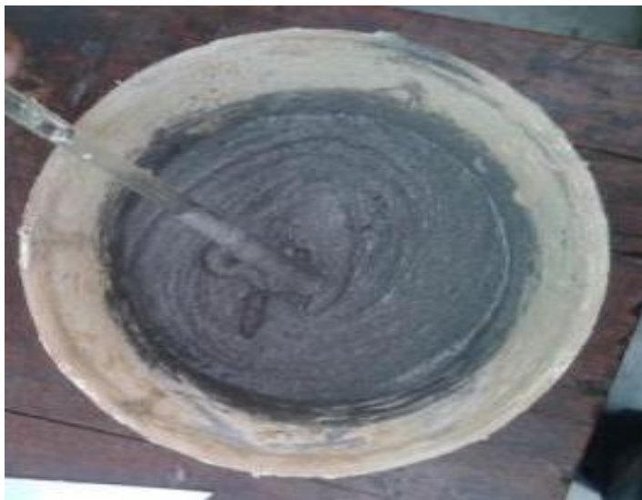
Figure 5.3: Media mixed with CNT and Al 2 O 3 abrasive particle
