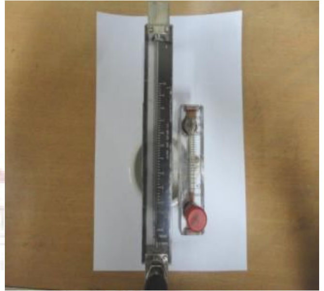
Figure 3.5.4 Rotometer fitted at Air nozzle for measuring air mass flow
