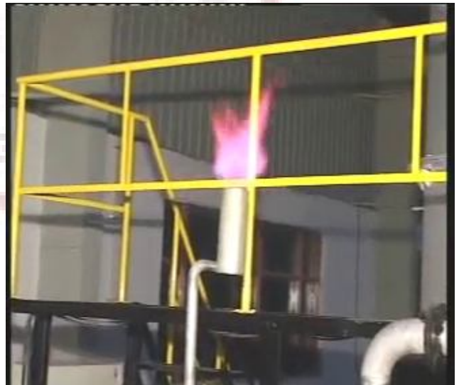
Figure 3.5.5 Gasifier Running at Flare mode
