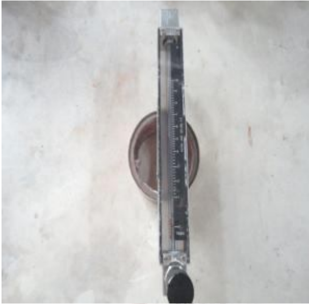
Figure 3.5.4 Rotometer fitted at Air nozzle for measuring air mass flow
