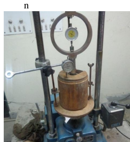
Figure 36: testing of CBR specimen
