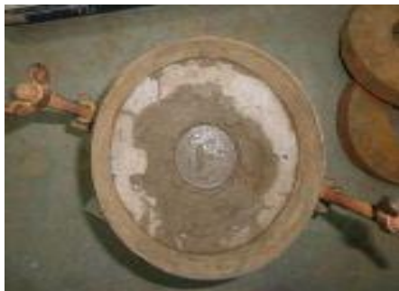
Figure 35: Sample prepared in CBR mold
