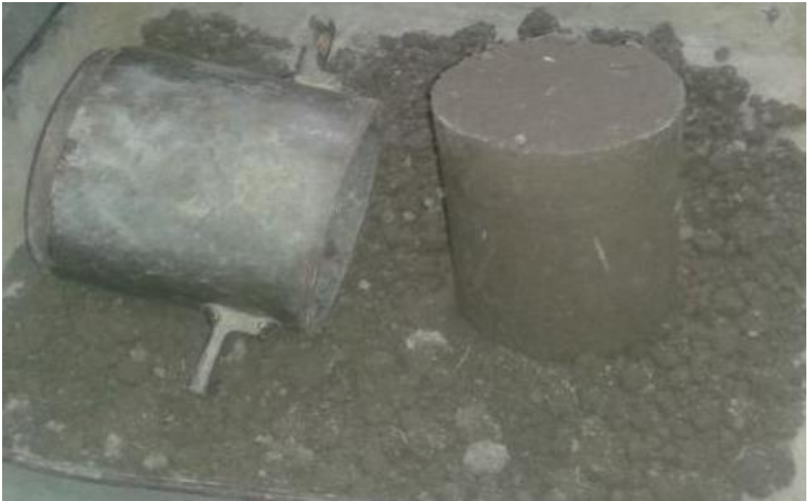
Figure 26: Sample prepared in standard proctor test
