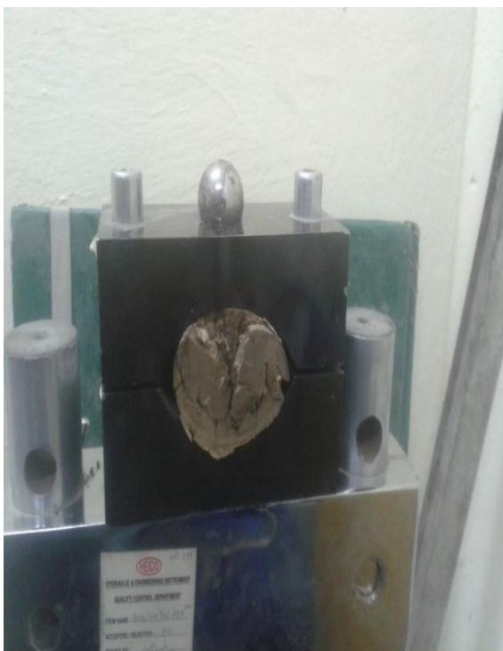
Fig.69: Complete Failure at 14 days
