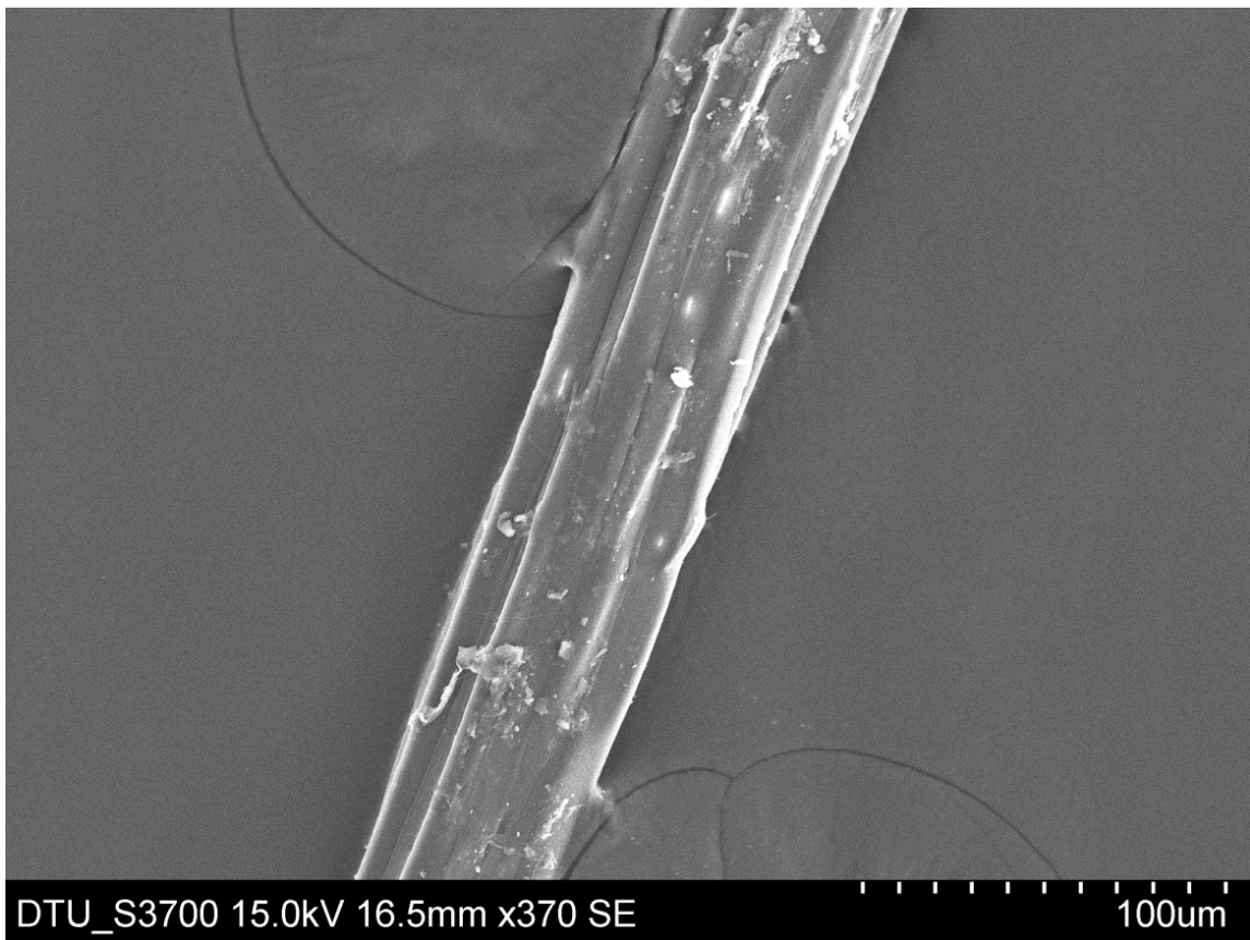
Fig.18: Jute Fibre at 100um scale
