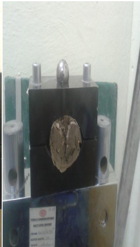
Fig.68: Failure of Sample at 7 days curing
