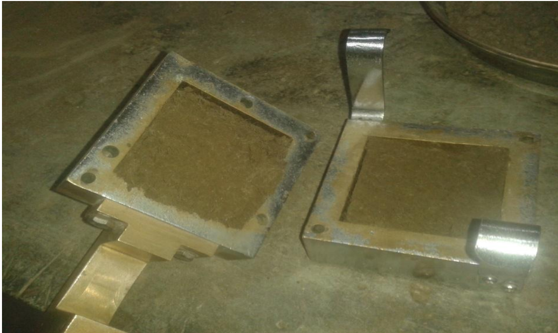
Fig.82: Failure of Sample at 10KN/m 2
