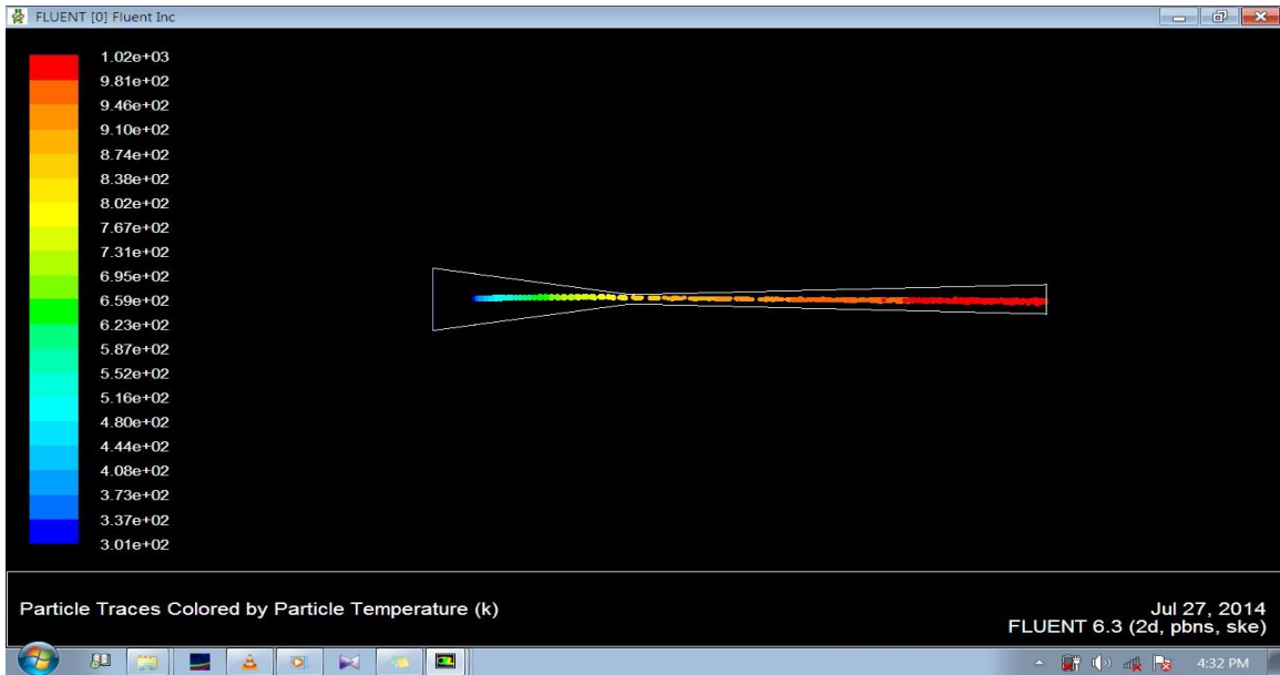
Fig.14a. Figure shows that maximum Temp. of Particles at outlet of the nozzle is 1002^{\circ}K
