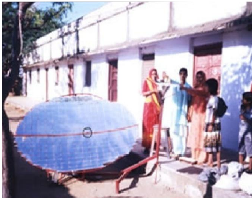
Fig. 4.5 : Manual changing of length of the reflector's rear support for seasonal adjustment
