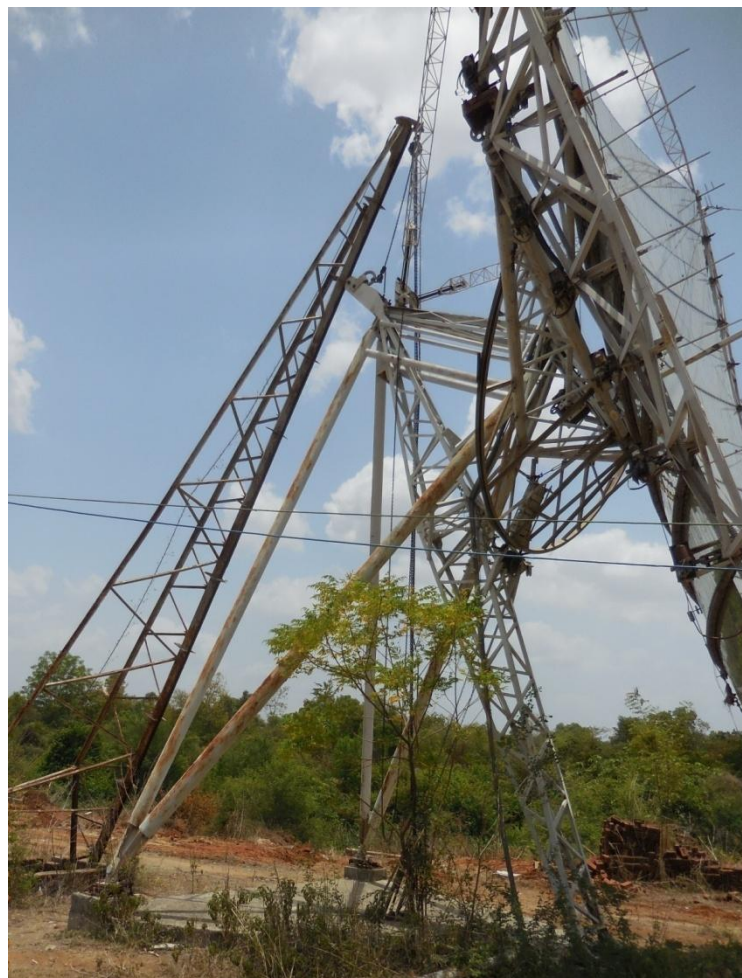
Fig. 4.4 : Crematorium tracking stand aligned with back crane and reflector frame
