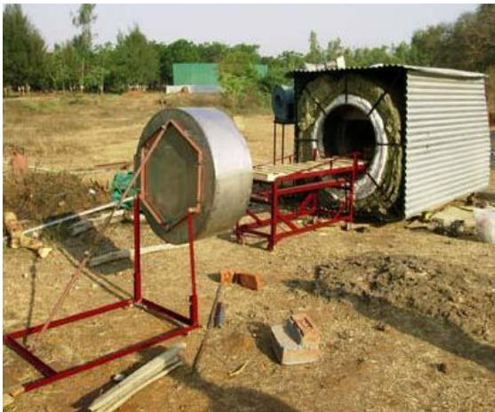
Fig. 4.12 : Chamber (back-side) with wooden bier on trolley & insulated "Closing Door"
