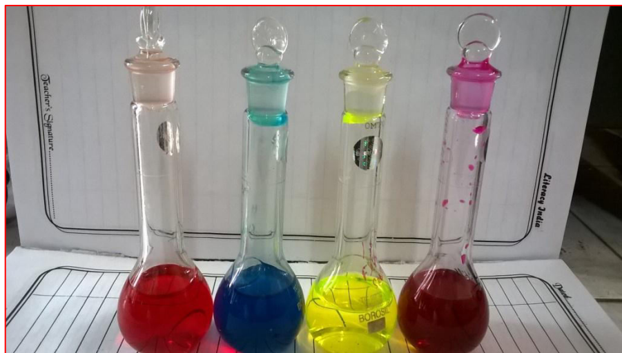
Figure 4.1 Prepared stock solution of different dyes in our laboratory.(a) Congo- red(b) Malachite green(c) Fluorescein sodium(d) Rhodamine b.
