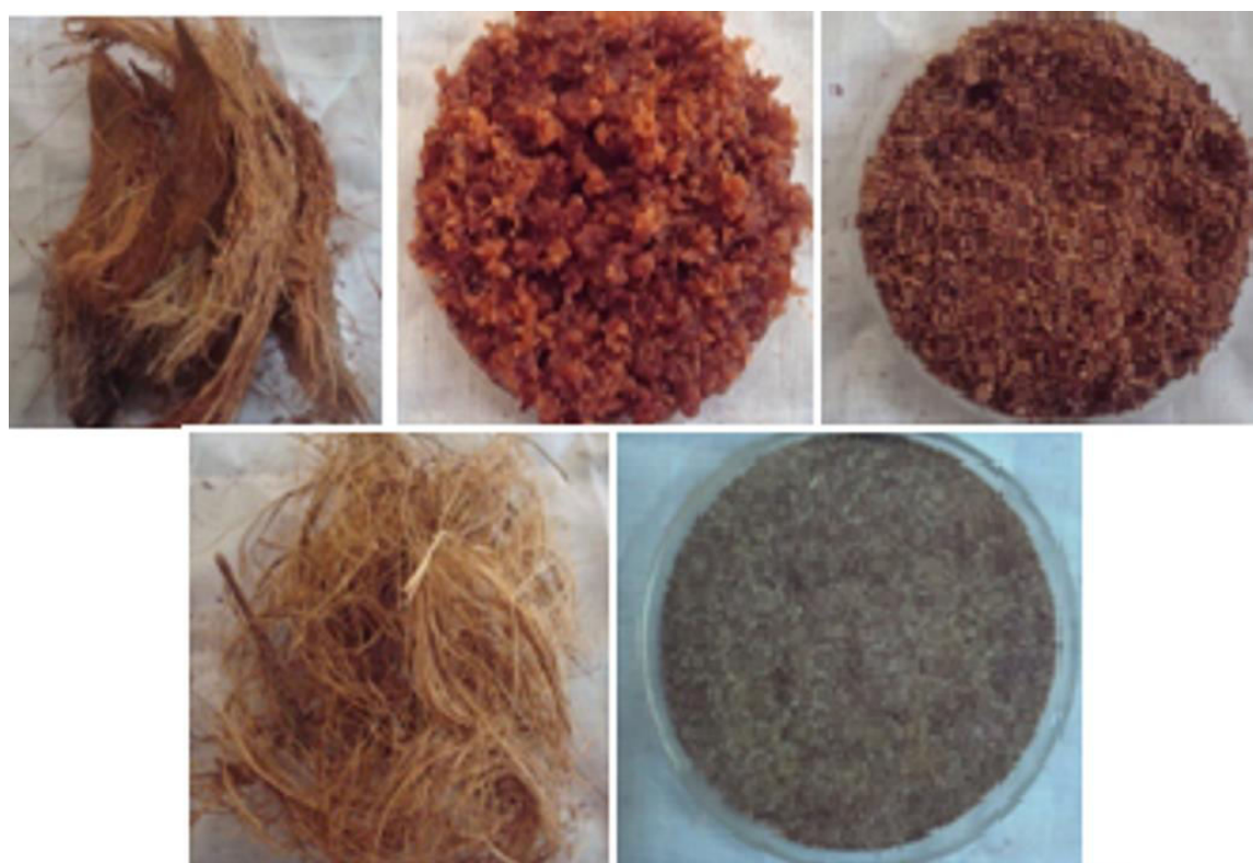
Figure 3—[a] coir husk [b] wet coir pith [c] dried coir pith [d] coir fibre [e] autoclaved coir pith
