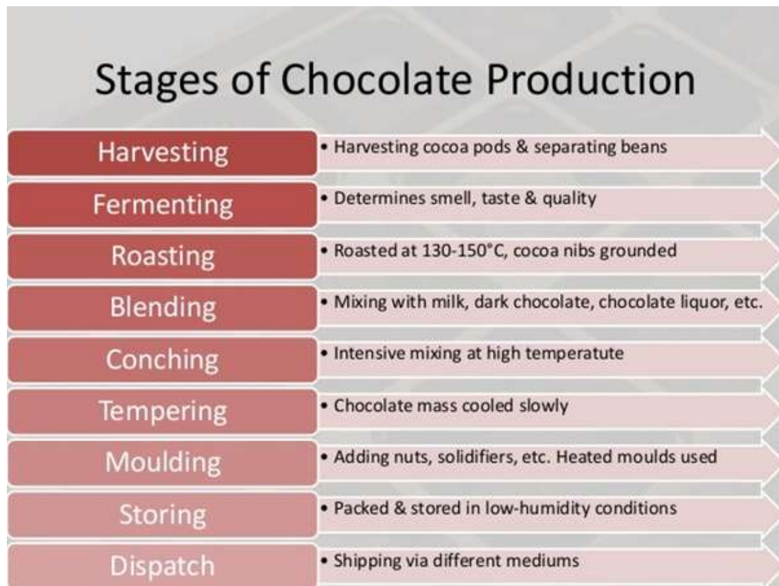
Figure 1: A composite flow diagram of the major operations for processing of the common chocolate products.
