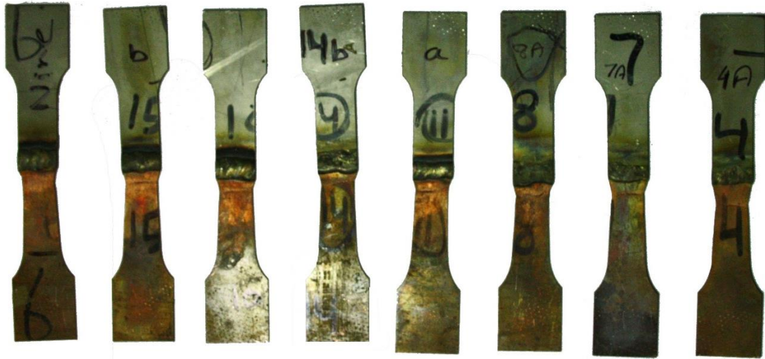
Figure 5. 10: Specimen after tensile test
