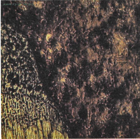
Figure 7. 7: Microstructure at fusion zone showing structure consisting of dendrites in a matrix of copper
