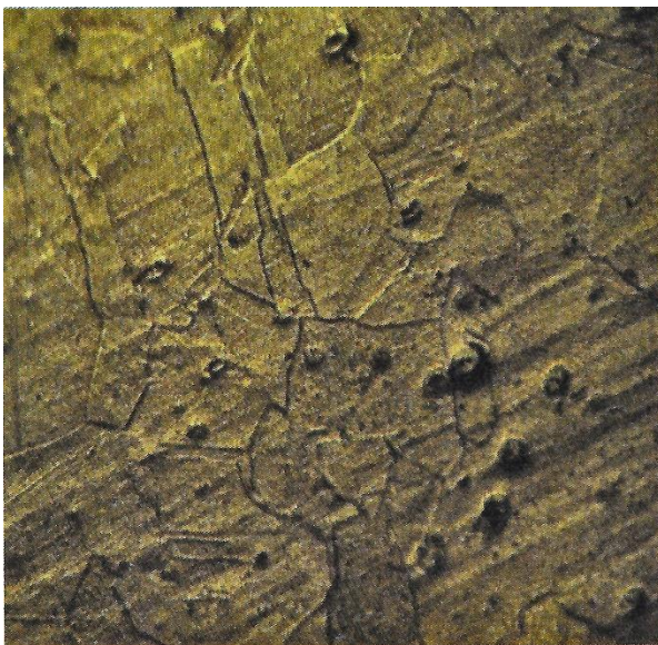
Figure 7. 5: Microstructure at heat affected zone, showing \alpha -phase with annealing twins
