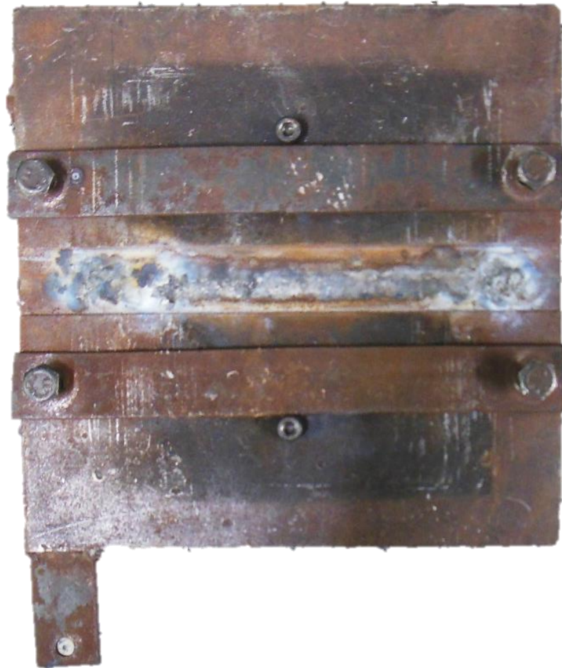
Figure 4. 7: Welding plate with work piece clamping strips
