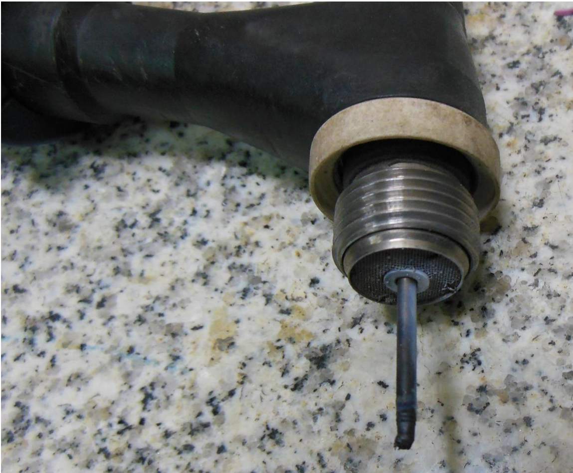
Figure 3. 5: Tungsten non consumable electrode
