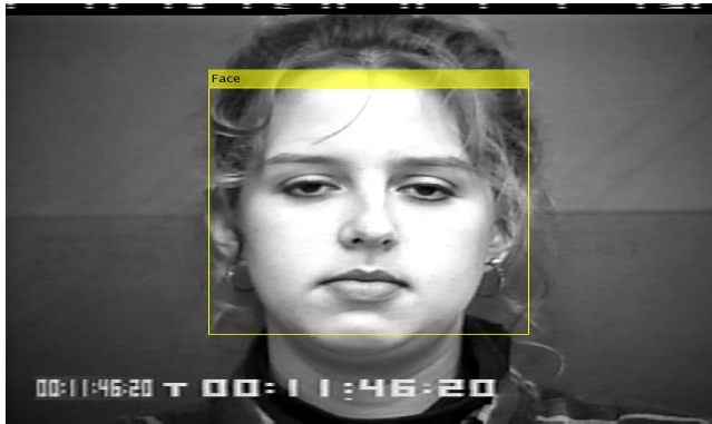
Fig 5.3.1.1: An example of Face Detection using Viola-Jones Detector
