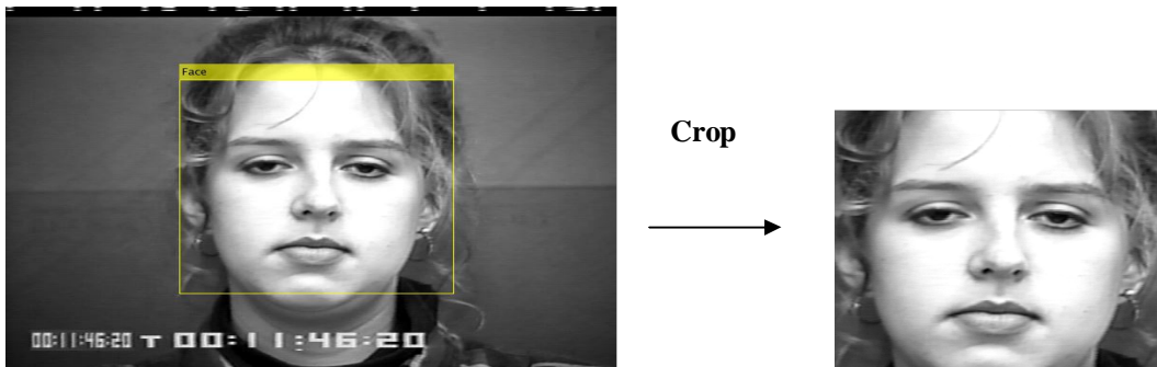
Fig 5.3.1.2: An example of Cropping the detected face
