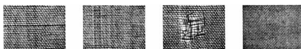
(a)Double yarn (b) Missing yarn (c) Broken Yarn (d) Variation of yarn
