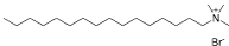
Figure 5.2: Structural diagram of CTAB
