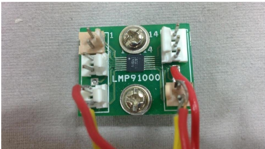
Fig3.3: Photograph of the lmp91000 IC mounted on a PCB
