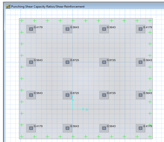
Fig-5.3.3.3: Punching shear values for various columns of flat plate thickened under column raft on soil-3 (i.e. Clayey Sand Silt with Gravels)
