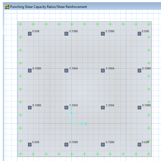
Fig-5.3.1.3: Punching shear values for various columns of flat plate raft on soil-3 (i.e. Clayey Sand Silt with Gravels)
