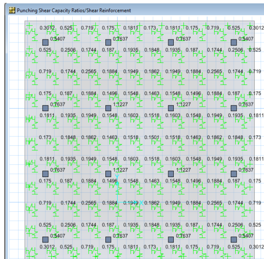
Fig-5.3.6.5: Punching shear values for various columns of pile raft on soil-5 (i.e. Sand-Silt mix with or without Gravel)
