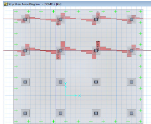
Fig-5.4.3.4: Shear force diagram of flat plate raft thickened under column for soil-4 (i.e. Sandy Silt)
