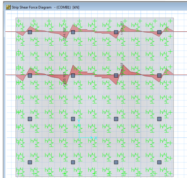
Fig-5.4.6.6: Shear force diagram of pile raft for soil-6 (i.e., Hard Mooram with Kanker)
