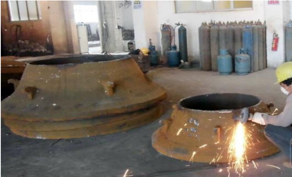
Fig. 4.7 Trimming and grinding [15]
