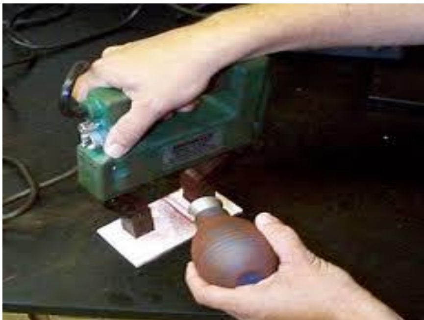
Fig.3.6 Magnetic particle inspection [15]
