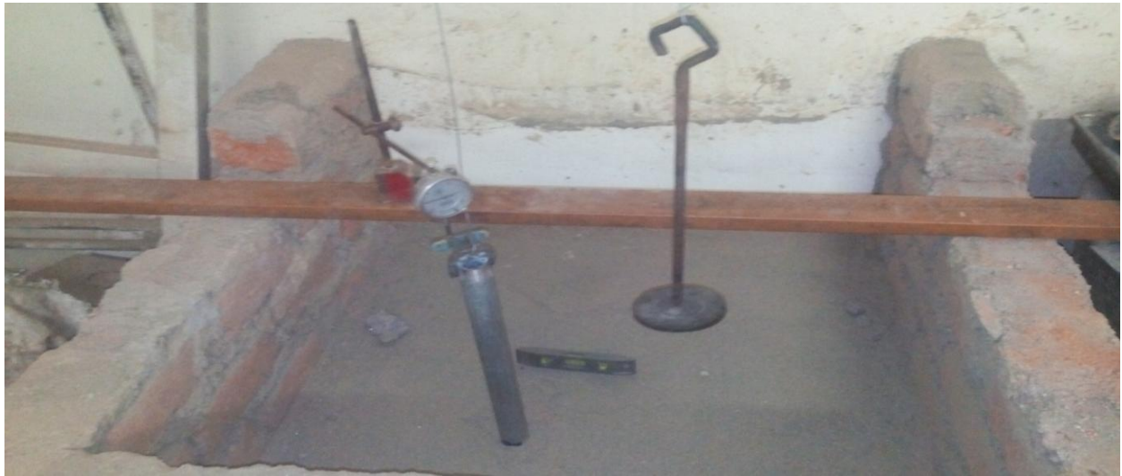
Fig 5 experimental set up for pull out test.
