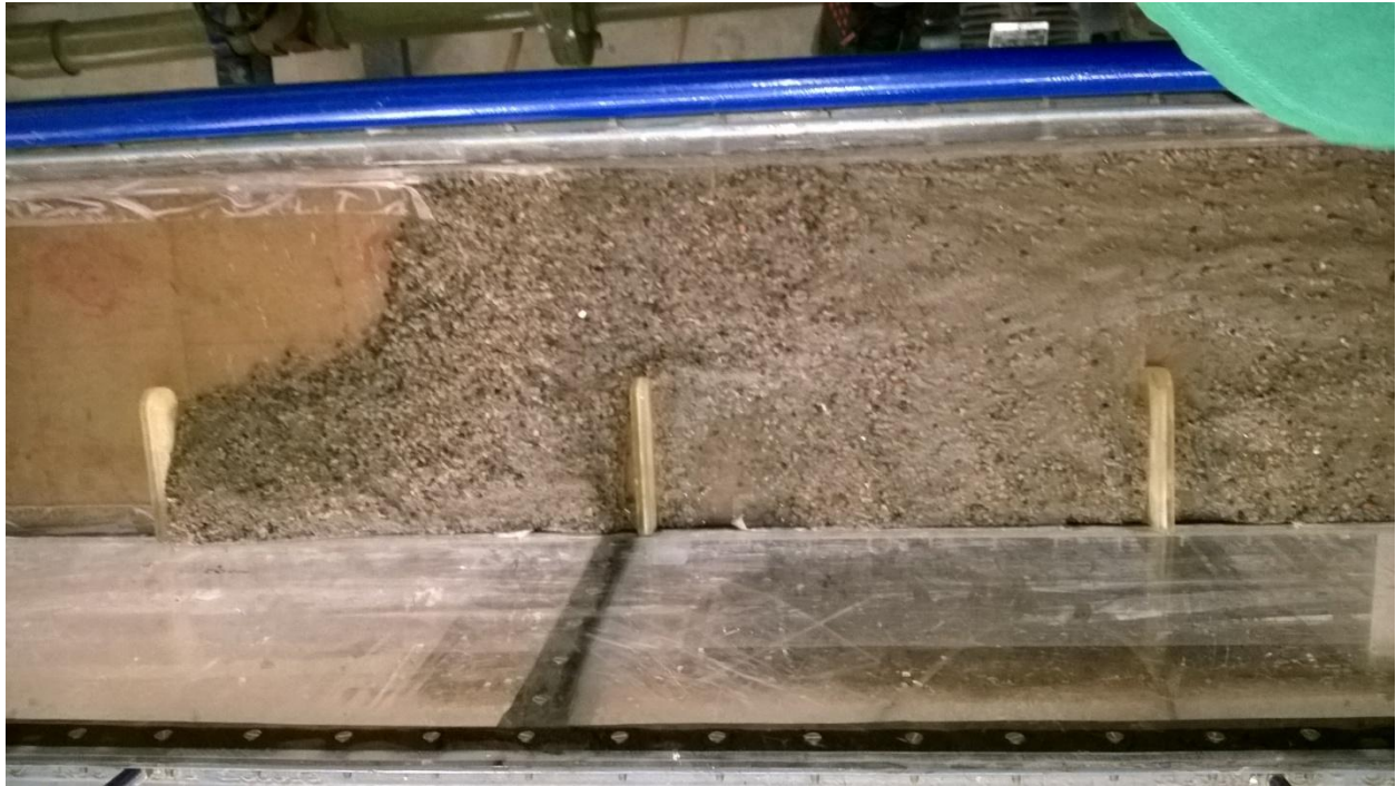
Fig 4.23: View of Sand bed after test on Groynes with depth of sand initially 1.5cm
