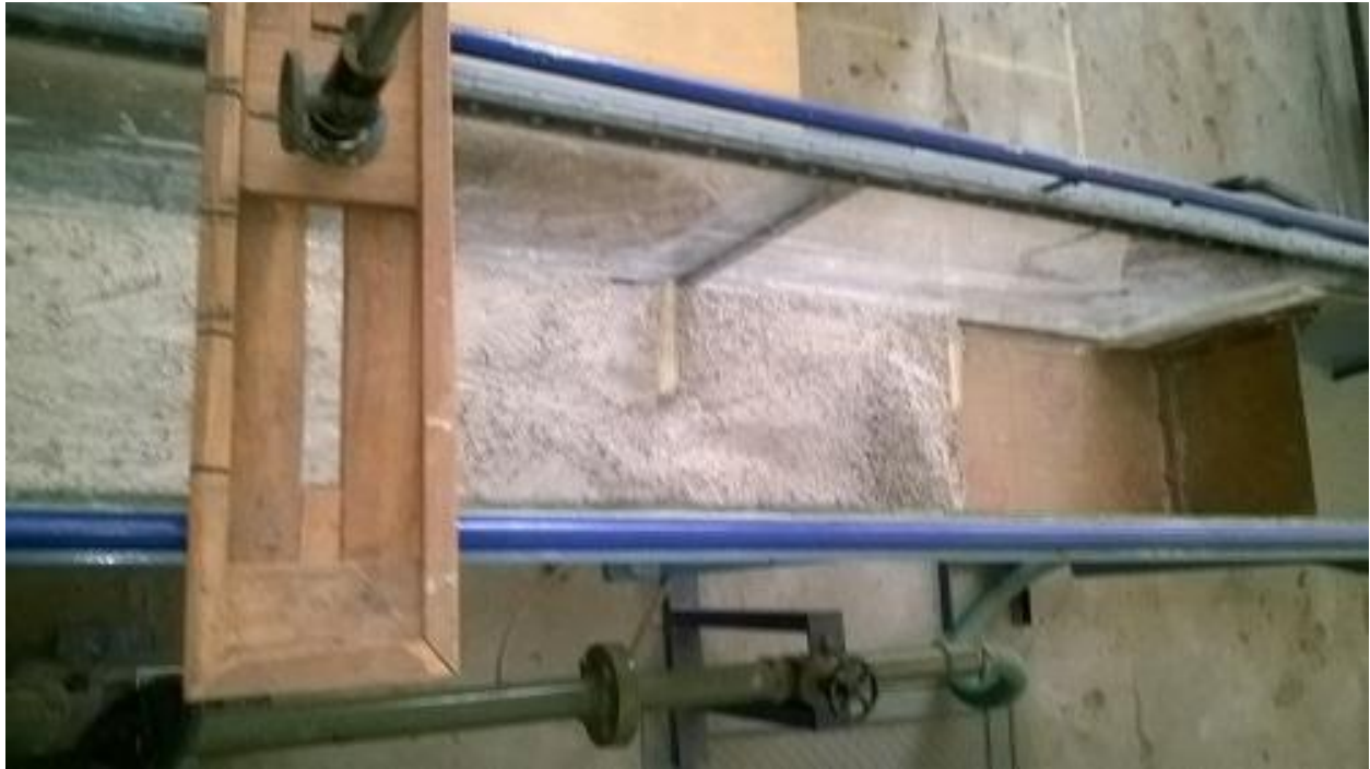
Figure 4.18: Dry River Bed of Flume after flow has taken place for Case 2(b)
