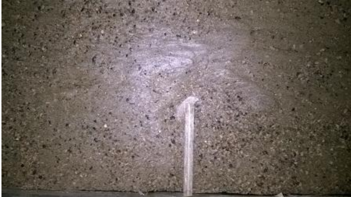
Figure 4.30 Bed form Developed near Groyne tip for Case 3(a)
