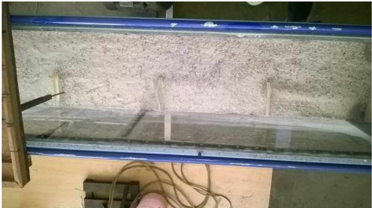
Figure 4.13: View of dry River Bed of Flume after flow has taken place for Case 2(b)
