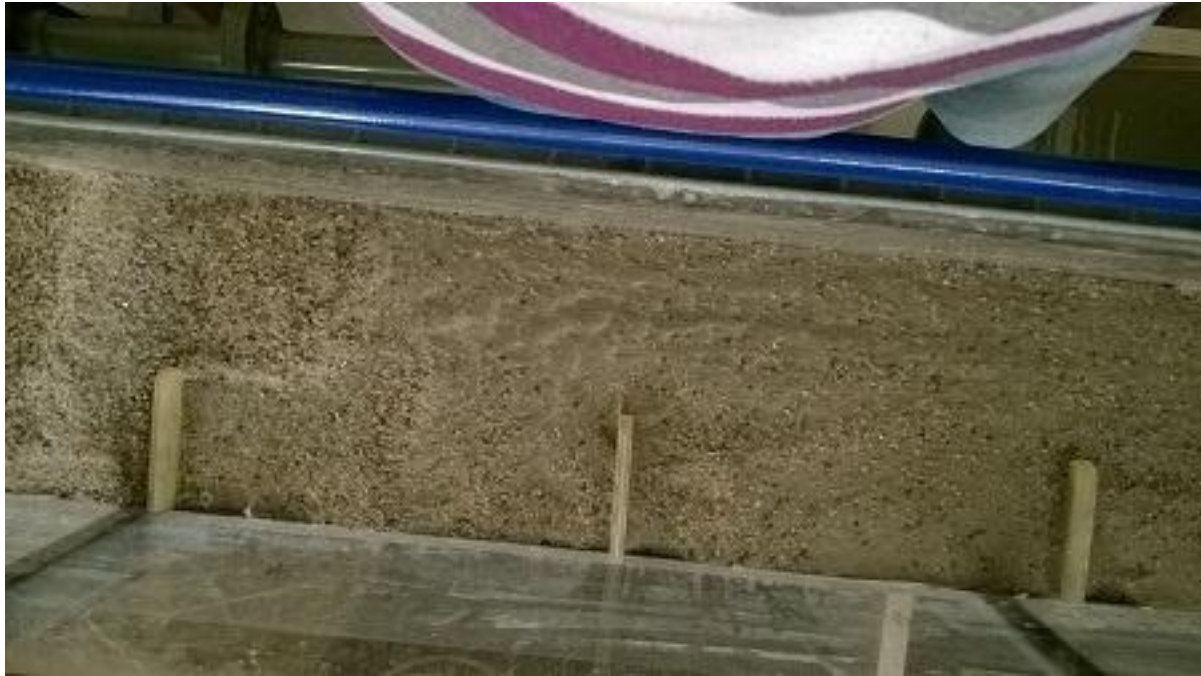
Fig. 4.38: Formation of Scour Holes near Groyne tip for case 3(a)
