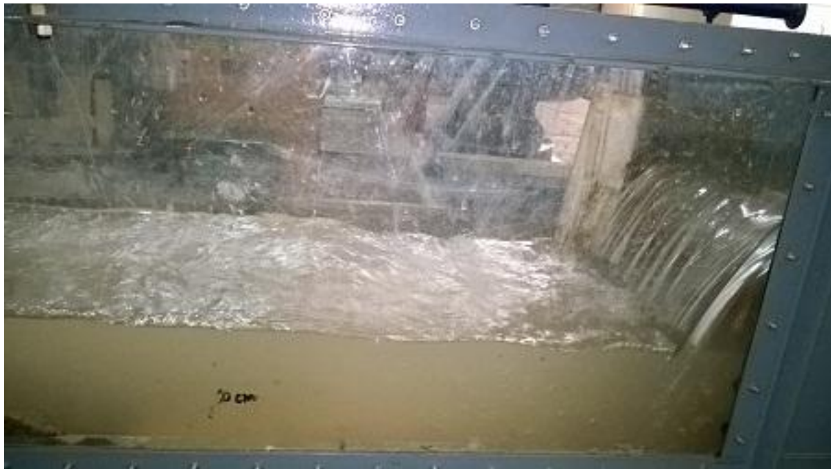
Fig 4.36: Turbulence created in the flow by upstream currents for case 3(c)
