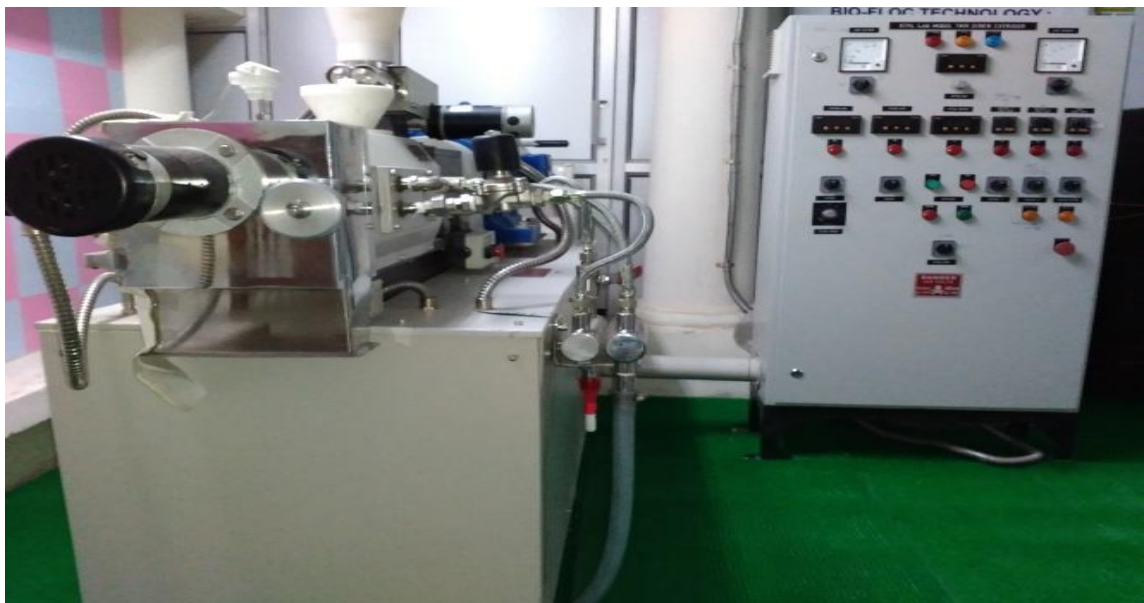
Fig. 4. The feed making unit, (a) Twin screw extruder (b) Panel board
