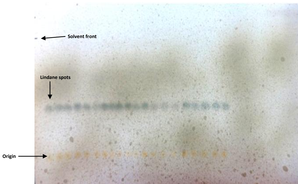
Fig. 4.5 TLC plate of degradation of lindane by consortium
