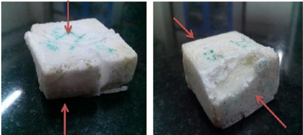
Fig 3.20: The photographs of compression tested samples (a) perpendicular, (b) parallel are presented (arrows indicate direction of loading)
