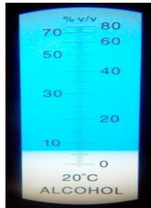
FIGURE 14: Alcohol response on an alcohol refractometer
