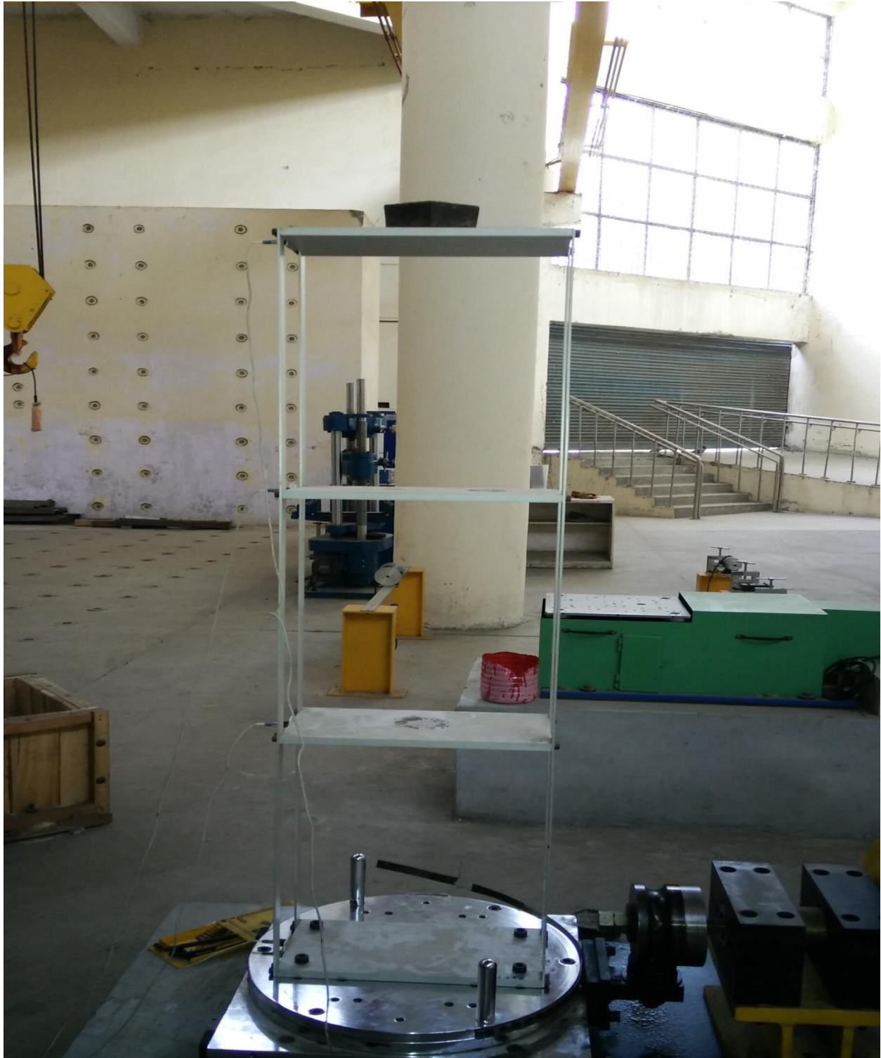
Fig. 5.12 model with additional mass on 3 rd floor
