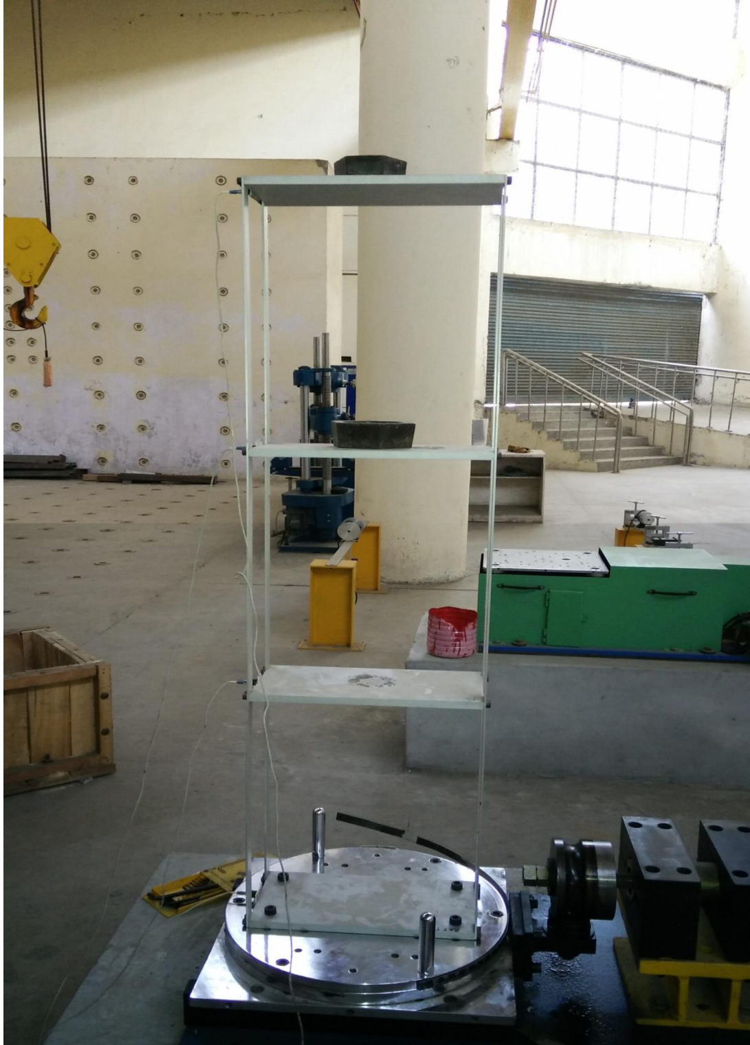
Fig. 5.16 model with additional mass on 2 nd floor and 3 rd floor
