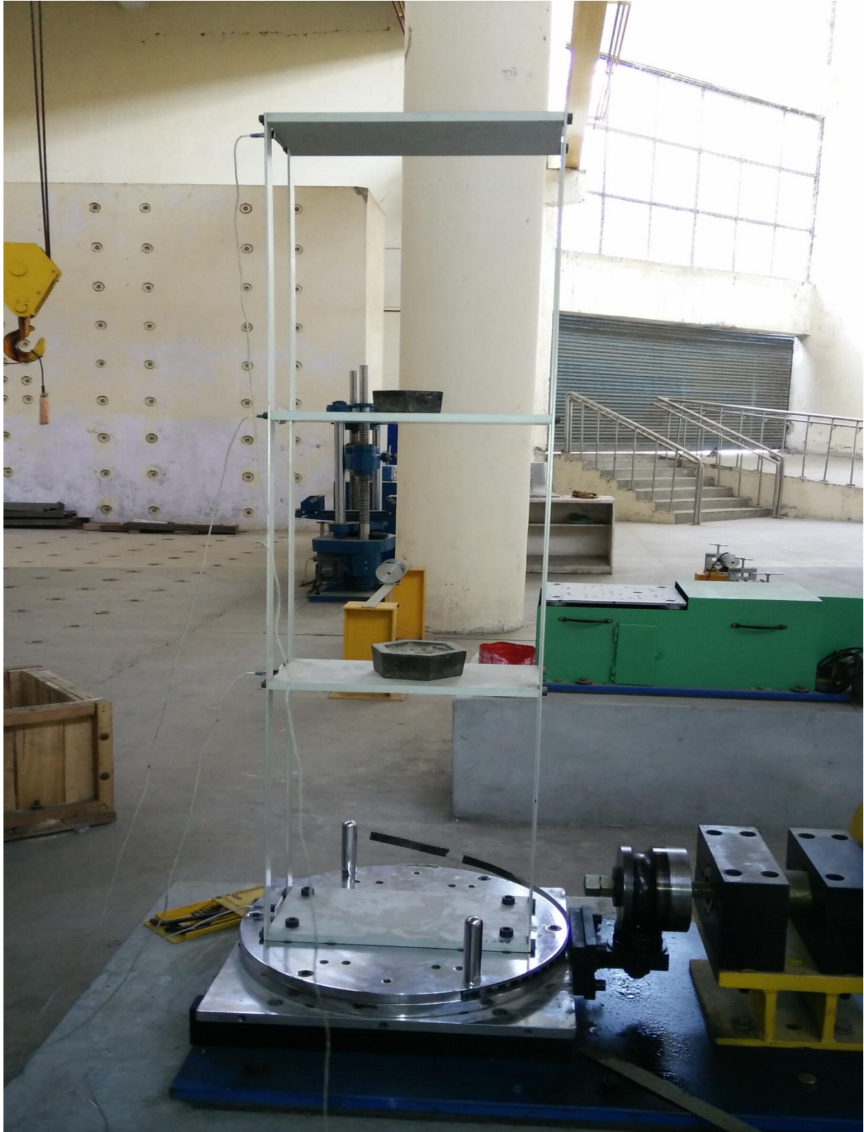
Fig 5.14 model with additional mass on 1 st and 2 nd floor
