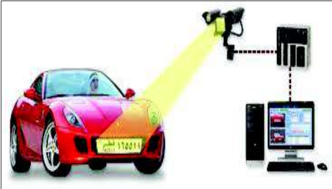
Figure 3: number plate detection, tracking and recognition in each video frame [Source: www.getti-images]
