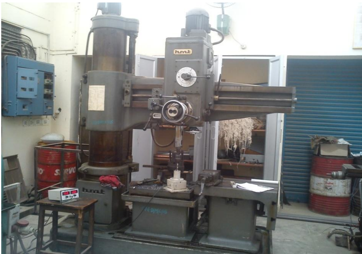
Fig.3.3. A TYPICAL RADIAL DRILLING MACHINE IN METAL CUTTING LAB, DTU NEW DELHI
