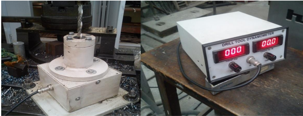
Fig.3.4.DYNAMOMETER SETUP USED IN THE PROCESS AT METAL CUTTING LAB, DTU
