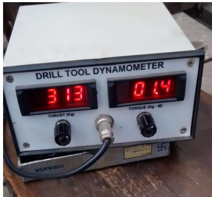
Figure 6 : dynamometer used in the process at metal cutting lab, dtu
