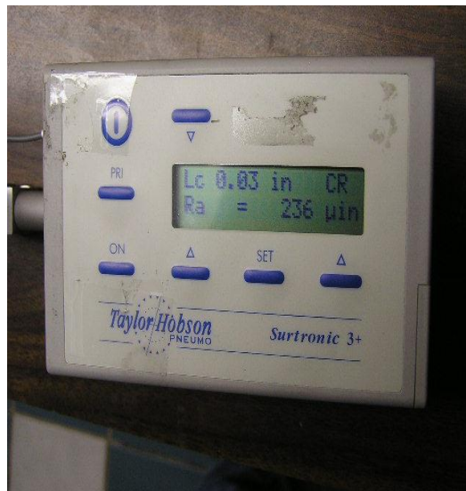
Figure 7 : a taylsurf instrument by taylor hobson surtonic 3+ at metrology lab, dtu
