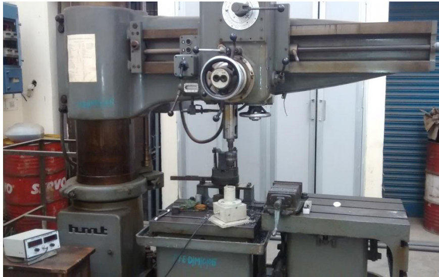
Figure 4: drilling machine used in process at metal cutting lab, dtu
